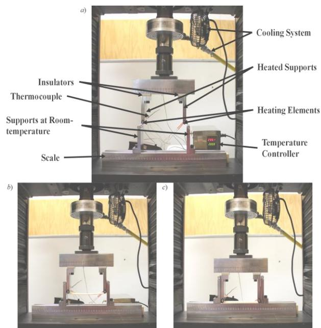
Fig. 2. Representation of a) the experimental setup, b) the rig during the experiment and c) the rig when the supports have reached the final position before retraction.
