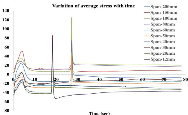
Fig. 4. Variations in the stresses experienced due to changing the span lengths of the plywood from 200 mm to 12 mm.
