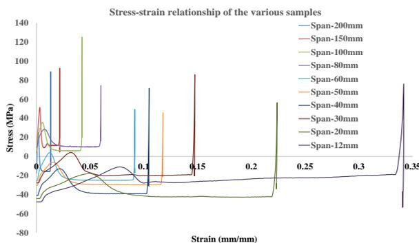
Fig. 5. Stress-strain analysis of the various span lengths of the plywood from 200 mm to 12 mm.
