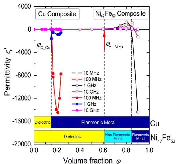
**Fig. 6.** Real part of permittivity  $\epsilon_r'$  for the  $\text{Ni}_{47}\text{Fe}_{53}$  composites as a function of the particle volume fraction  $\varphi$ . The  $\varphi_c$  denotes electrical percolation threshold.
