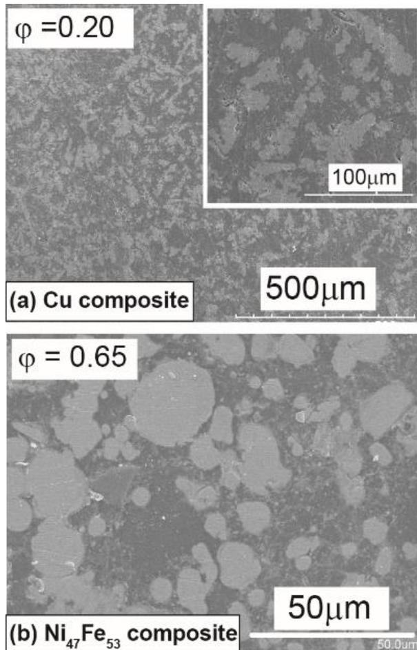
**Fig.1.** Scanning Electron Microscope (SEM) images of the polished surface of Cu and Fe<sub>53</sub>Ni<sub>47</sub> composites (a) Cu:  $\phi = 0.20$ , (b) Fe<sub>53</sub>Ni<sub>47</sub>:  $\phi = 0.65$ ) [6, 9]
