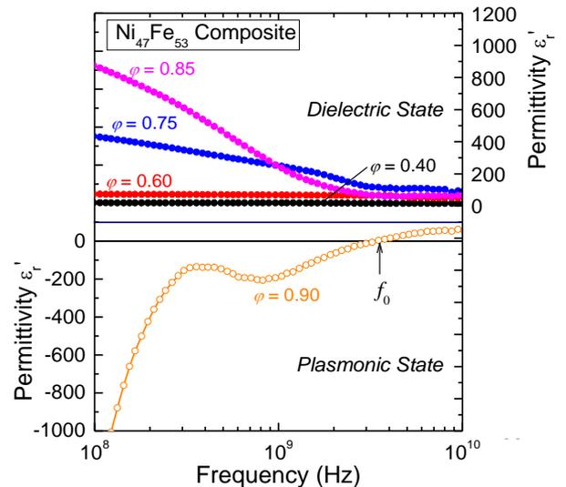
**Fig.4.** Real part of permittivity for  $Ni_{47}Fe_{53}$  composites at various  $\phi$  as a function of frequency. The  $f_0$  indicates the characteristic frequency in the plasmonic state.
