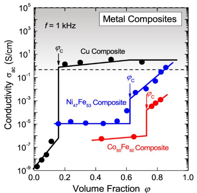
**Fig.2.** Electrical conductivity  $\sigma_{ac}$  of metal granular composite materials as a function of the volume fraction of particles. The dashed line indicates the boundary between non plasmonic and plasmonic state.
