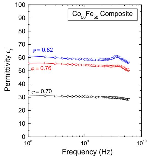
**Fig. 5.** Real part of permittivity for  $\text{Co}_{50}\text{Fe}_{50}$  composites at various  $\varphi$  as a function of frequency.
