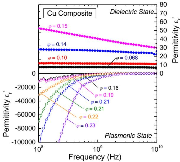
**Fig.3.** Real part of permittivity for Cu composite materials at  $\phi$  as a function of frequency.
