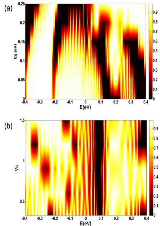
**Fig. 2.** (Color online) Contour plot of the electron transmission versus the incident energy  $E$  for (a) different barrier energy gaps,  $\Delta_B$ , (b) Fermi velocity ratio ( $v_c$ ).  $d_W = d_B = 50 \text{ nm}$  and  $N=15$ ,  $\Delta_B = 0.1 \text{ eV}$ .
