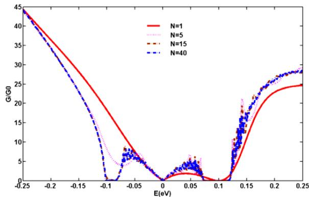
**Fig. 3.** (Color online) The effective conductance  $G^*$  as a function of incident energy for different  $N$ ,  $d_w, d_g = 50 \text{ nm}$ ,  $\Delta_g = 0.1 \text{ eV}$  and  $V_c = 1.3$ .
