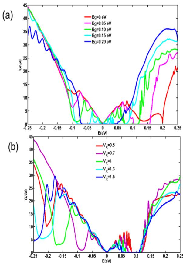
**Fig. 4.** (Color online) The effective conductance  $G^*$  as a function of incident energy for different (a) energy gap ( $\Delta_g$ ) and  $V_c = 1.3$ , (b) Fermi velocity ratio,  $\Delta_g = 0.1 \text{ eV}$ ,  $d_w = d_g = 50 \text{ nm}$ .
