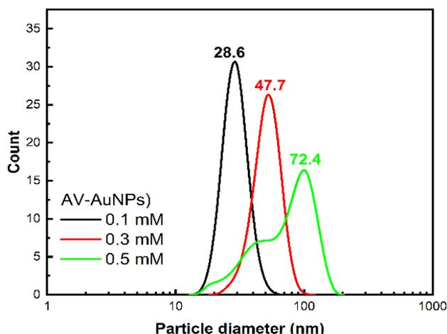
Fig. 4. Size distribution of AV-AuNPs with varying concentrations of gold precursor concentration. The increase in precursor concentration increased the hydrodynamic sizes of nanoparticles.
