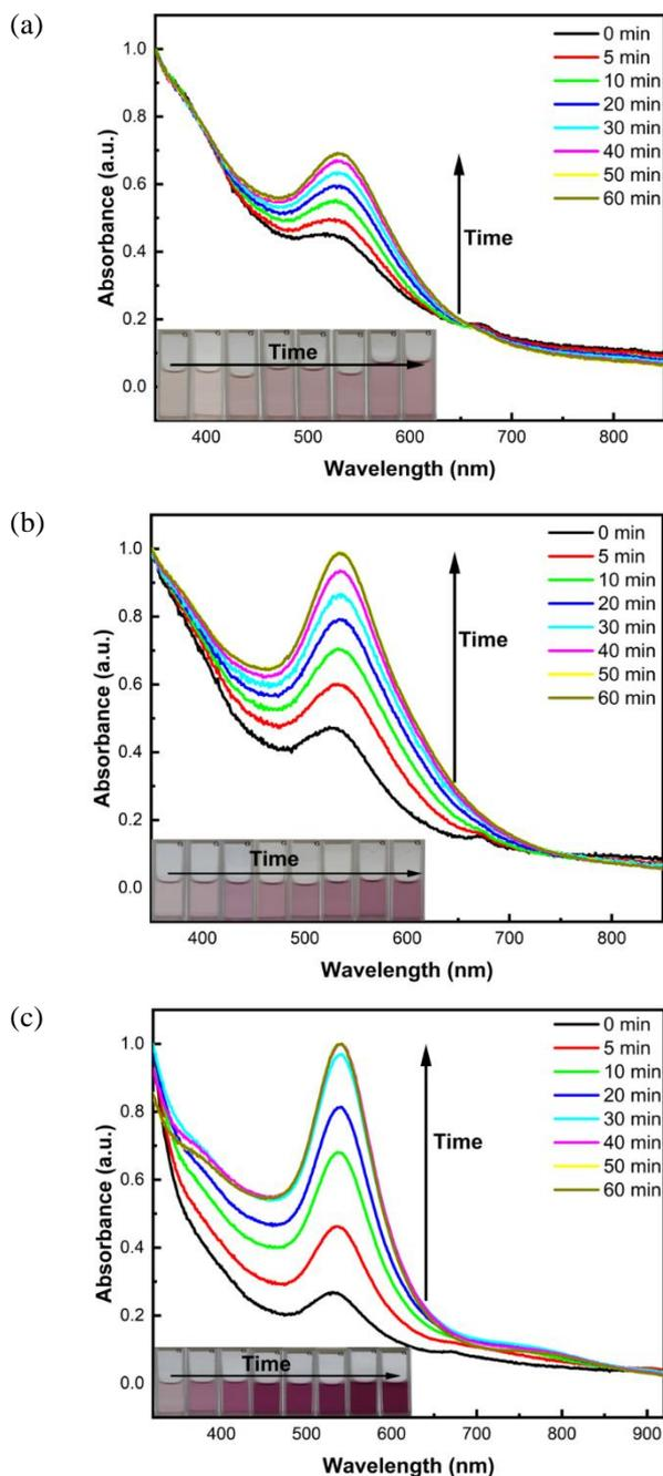
**Fig. 2.** UV-vis absorption spectra for the continuous growth of AV-AuNPs. Prepared by using (a) 0.1 mM, (S2) 0.5 mM, and (c) 0.5 mM gold precursor concentration. Experiments were performed at 60°C. The insets display the actual photographs of the AV-AuNP's growth within 1 h with different time intervals.
