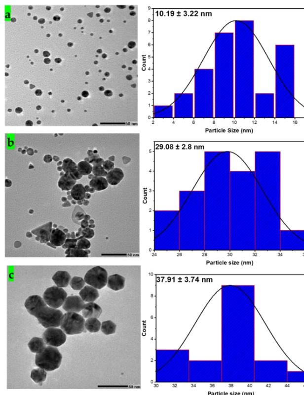
**Fig. 3.** (Left) TEM micrographs of AV-AuNPs at 50 nm scale prepared with (a) 0.1 mM, (b) 0.3 mM, and (c) 0.5 mM gold precursor. The shape of most NPs is spherical, while triangular and hexagonal shapes are also observed. (Right) Corresponding histogram of the particle size distribution.
