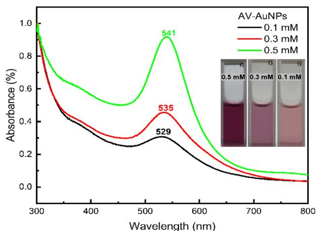
**Fig. 1.** UV-vis absorbance spectra of AV-AuNPs with varying gold precursor concentrations. The inset displays the actual photographs of AV-AuNPs.
