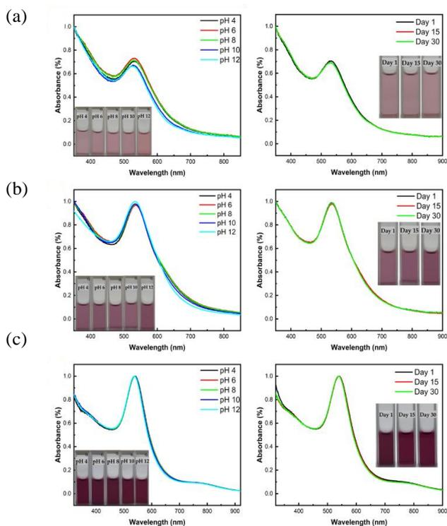
**Fig. 6.** (Left) UV-vis spectra of AV-AuNPs solutions recorded at 24 h with different pH values. (Right) Time-dependence stability study of AV-AuNPs stored at  $4^{\circ}\text{C}$  for various durations. (a) 0.1 mM AV-AuNPs; (b) 0.3 mM AV-AuNPs; and (c) 0.5 mM AV-AuNPs. All samples are stable across varied pH conditions and storage durations. The inset displays the actual appearance of AV-AuNP solutions.
