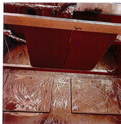
Fig. 12. EB-PVD system after the evaporation process
