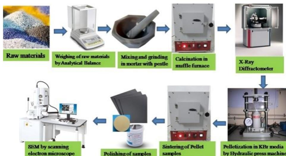
Fig. 1. Schematic diagram of solid state reaction method.
