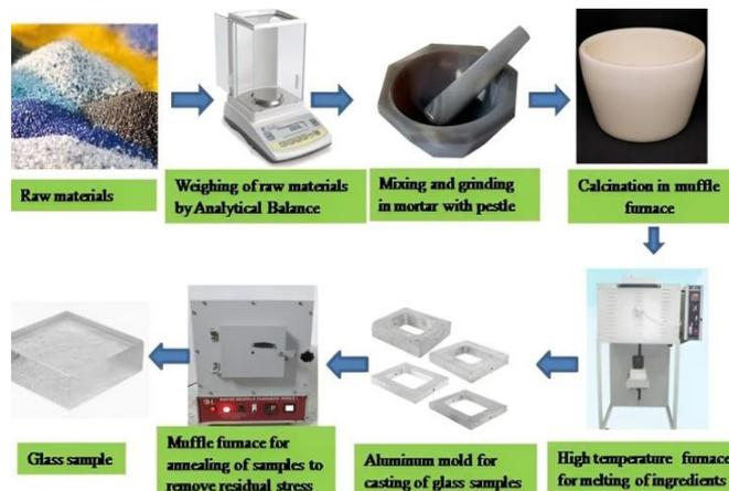
Fig. 5. Schematic diagram of melt quench method.
