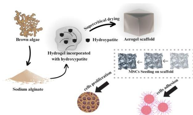
**Fig. 10.** A schematic illustration demonstrates the preparation and application of an alginate-based aerogel scaffold fabricated through 3D-printing and supercritical drying. This scaffold exhibits exceptional porosity, biocompatibility, and excellent fidelity to the CAD-pattern design, adapted from [226].
