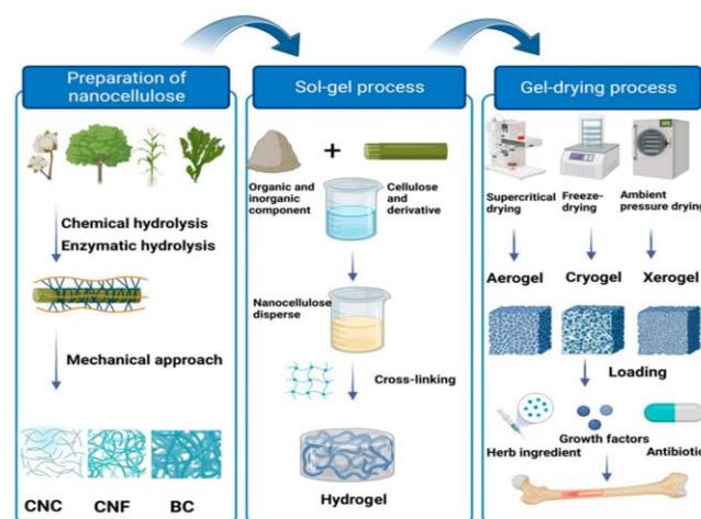
Fig. 9. Fabrication process of cellulose-based aerogels using the sol-gel method involves three main steps. First nanocellulose is prepared by purifying cellulose through chemical and enzymatic hydrolysis, followed by separation to form nanoscale cellulose materials using mechanical techniques. Second a sol-gel process takes place, where the polymer is dispersed in a solvent and undergoes a crosslinking stage. Third the gel-drying process is carried out [225].
