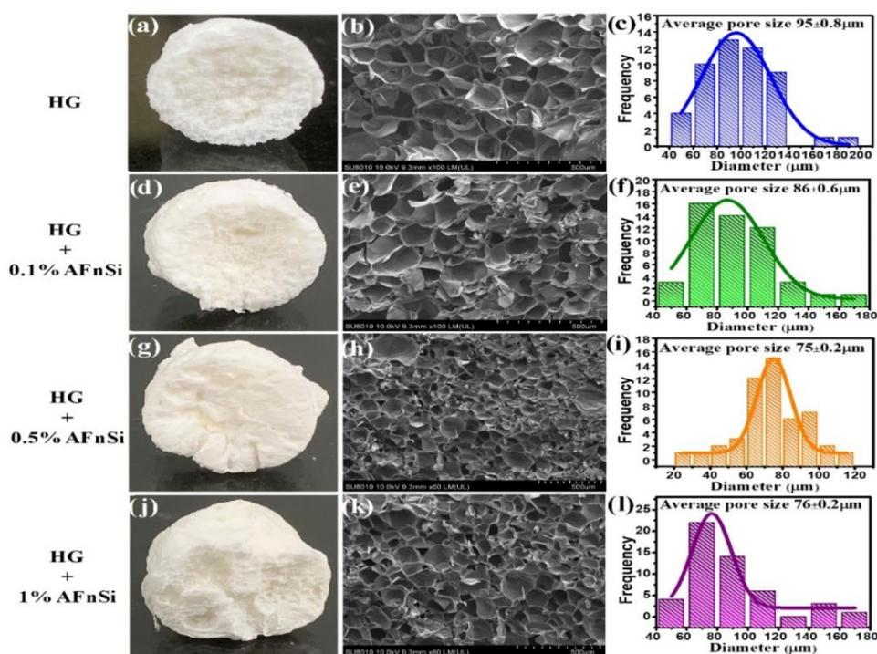
Fig. 7. Cross-sectional SEM picture of hybrid hydrogel scaffolds with various AFnSi concentrations along with its size distribution histograms [201].
