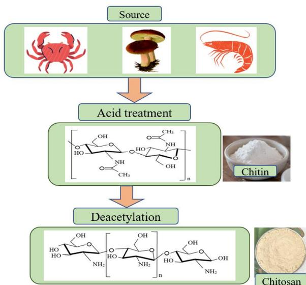
**Fig. 6.** The extraction of Chitosan from natural sources, such as crab shells, crustaceans, fungi, etc., consists of two main steps: acid treatment and deacetylation.
