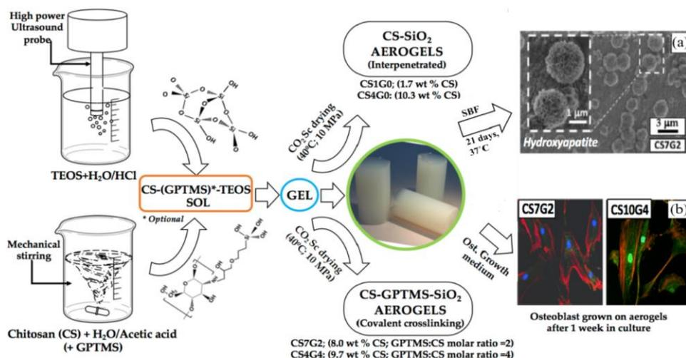
**Fig. 8.** Illustration and preparation of novel synthesis route for obtaining homogeneous chitosan (CS)-silica hybrid aerogels showing SEM micrograph and Live/Dead staining of osteoblasts culture to evaluate the viability and compatibility of the aerogels [215].
