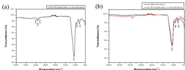
Fig. 7. (a) FTIR PA spectra; (b) FTIR PA and membrane spectra  $\mu$ Raman spectroscopy.
