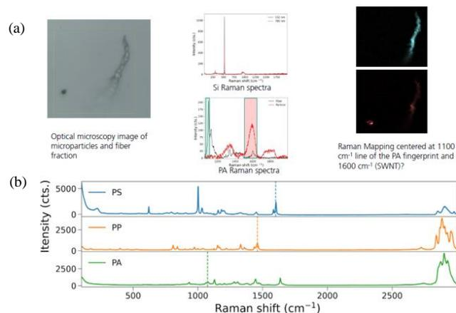
Fig. 8. (a)  $\mu$ Raman spectra; (b) standard spectra.
