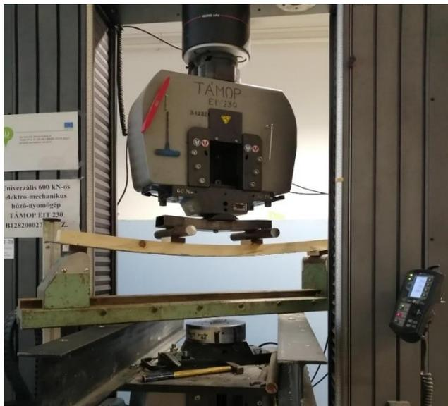
Fig. 2. Four-point bending test.
