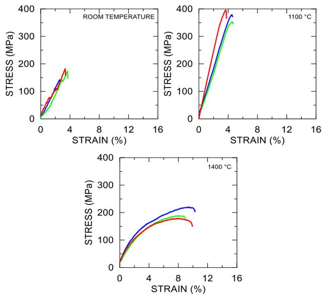
**Fig. 3.** Effort curves vs. deformation of SiC/Si composite evaluated in thermomechanical tests at (a) room temperature, (b) 1100 °C and (c) 1400 °C.
