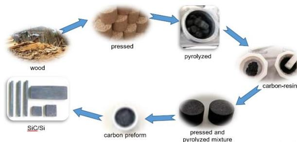
SiC/Si composites were manufactured using waste from the wood industry, sawdust was pressed in a 30 mm diameter metal steel mold and subsequently the pressed sawdust was subjected to a pyrolyzation process, up to temperatures of 800 °C for 1 hour.
