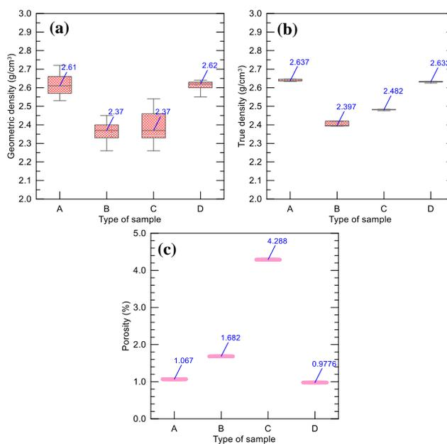
**Fig. 1.** Values of: (a) geometric density, (b) real density and (c) porosity for SiC/Si compounds studied.
