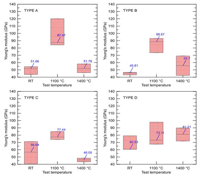
**Fig. 5.** Young's modulus values as a function of test temperature for SiC/Si compounds (a) type A, (b) type B, (c) type C and (d) type D.
