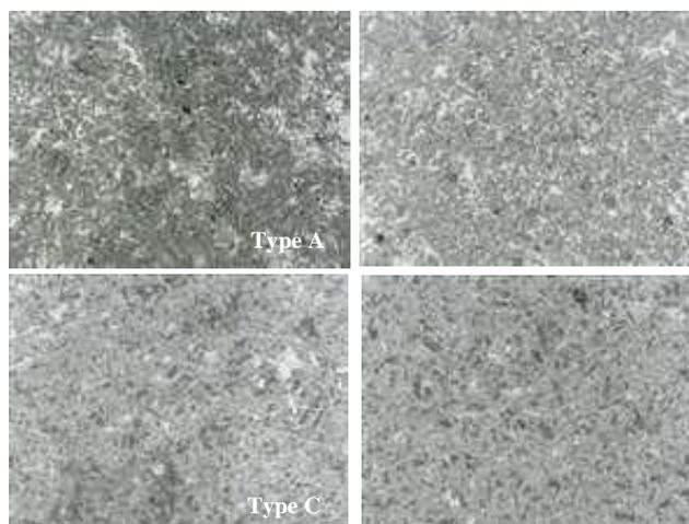
**Fig. 2.** Optical microscopy micrographs for the SiC/Si compounds studied.
