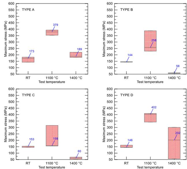
**Fig. 4.** Maximum strength values as a function of test temperature of SiC/Si compounds (a) type A, (b) type B, (c) type C and (d) type D.
