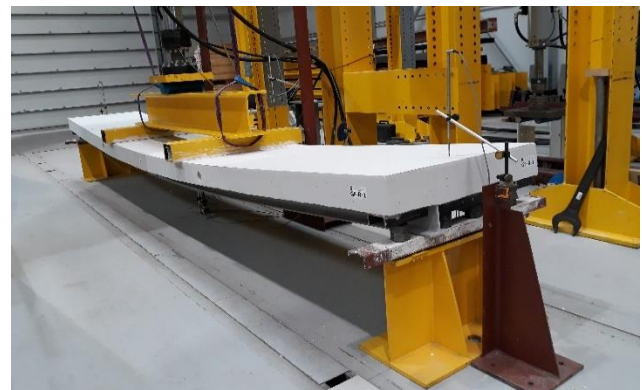
Fig. 4. Composite beam during the loading test.
