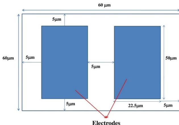
**Fig. 1(B)** Tunnel diode test structure area is  $60\mu\text{m} \times 60\mu\text{m}$ , while top electrode dimension is  $50\mu\text{m} \times 22.5\mu\text{m}$ .
