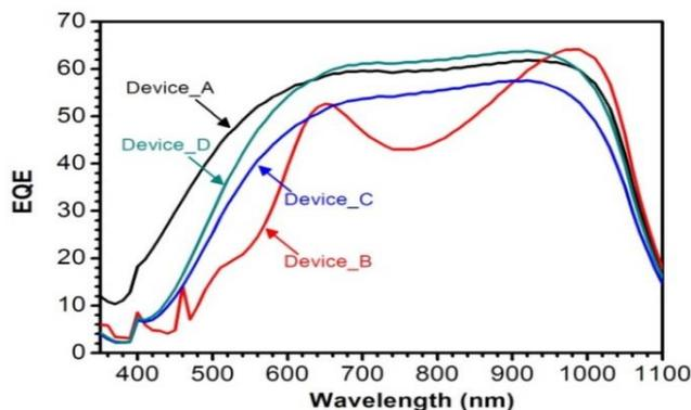
**Fig. 7.** External quantum efficiency spectra of silicon solar cells with and without tunnel layer as well as with an electron transport layer (TiO<sub>2</sub>).
