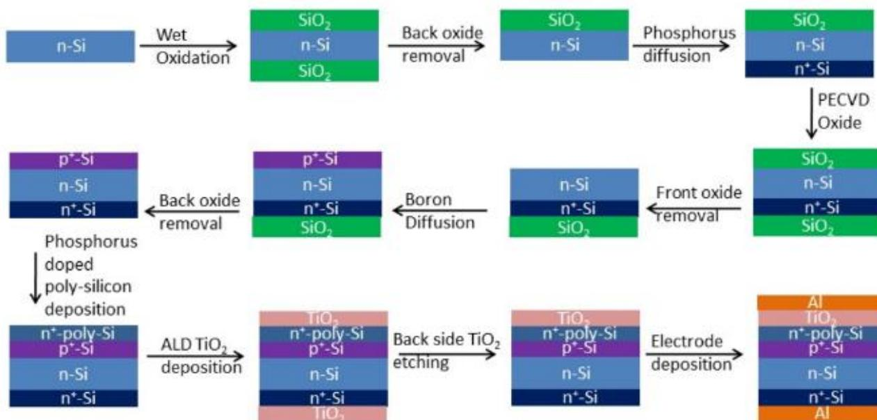
**Fig. 2.** Fabrication steps of the poly-silicon/c-silicon tunnel diode-based solar cells.
