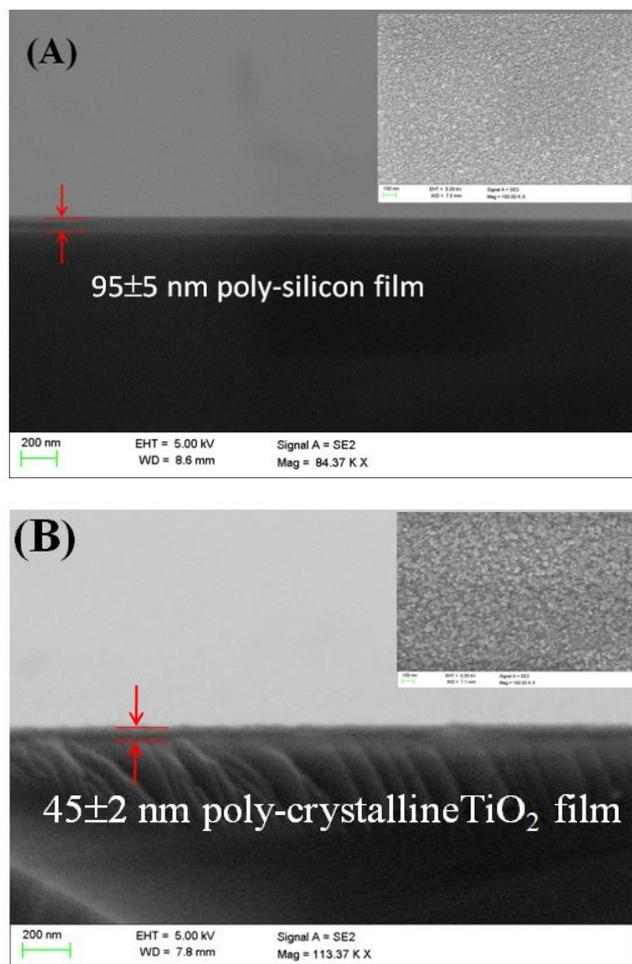
**Fig. 5.** Cross-sectional SEM images of (A) 95±5 nm thick poly-silicon film and (B) 45±2 nm thick polycrystalline TiO<sub>2</sub> film.
