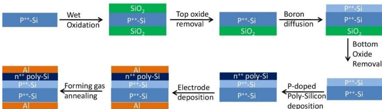
**Fig. 1(A)** Fabrication steps of the tunnel diode test structure.
