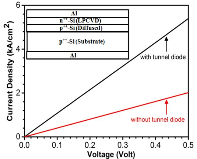
**Fig. 4.** J-V characteristics of the devices with and without tunnel diode (just substrate, Al/p<sup>+</sup>-Si/Al).
