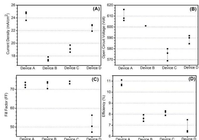
**Fig. 8.** Performance of various solar cells (3 cells in each group) in terms of (A) short circuit current density, (B) open-circuit voltage, (C) Fill-Factor, and (D) efficiency.
