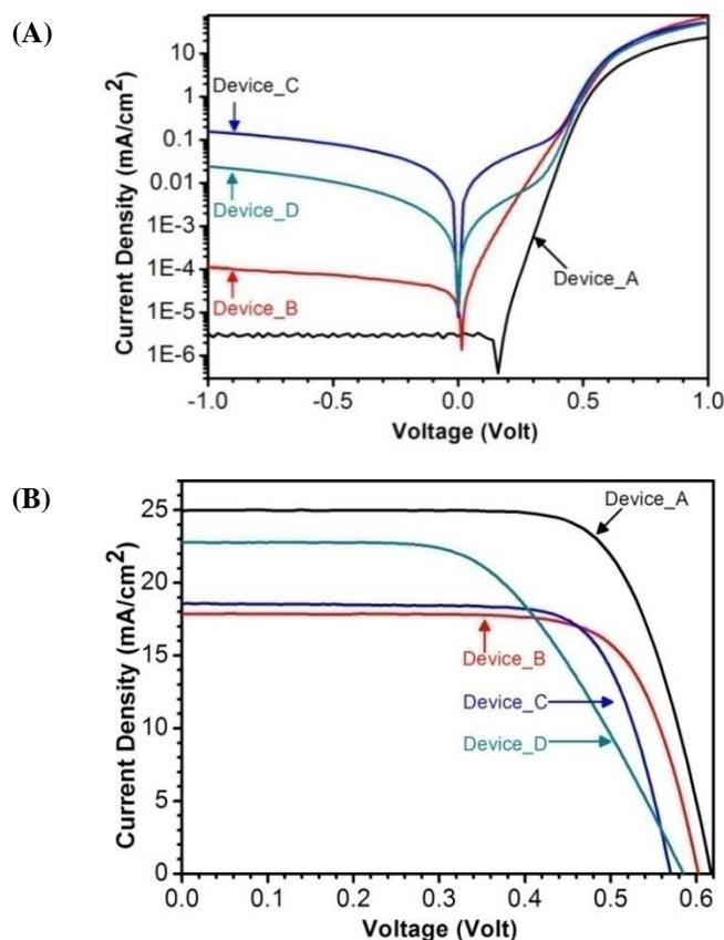
**Fig. 6.** J-V characteristics of as-fabricated solar cells: (A) in dark and (B) under AM 1.5G.
