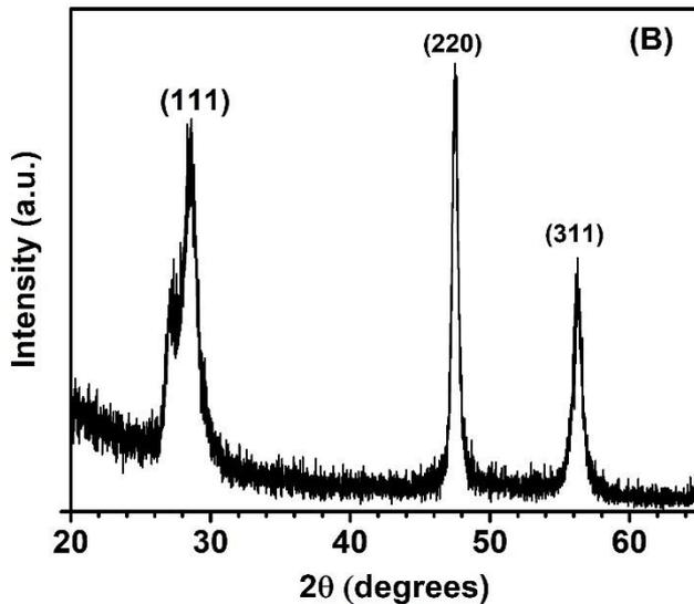
**Fig. 3.** (A) SEM images of a 195±10 nm thick poly-silicon film, (B) XRD pattern of poly-silicon film.
