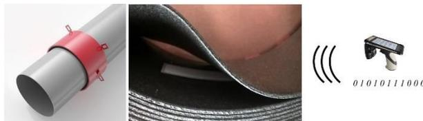
Scheme of identification process of a pipe collar with swelling anti-fire composite material with the use of RFID technology
