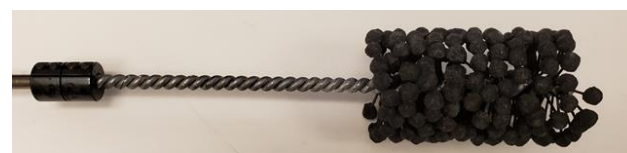
(d) Hone used to clean the inside of the ceramic tube.
