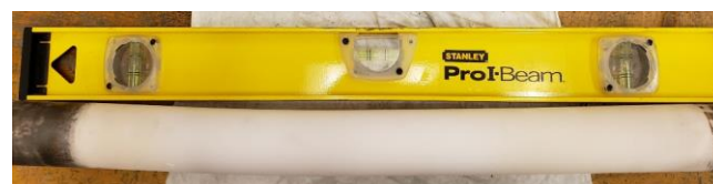
(c) A 24-inch long thick wall alumina tube (OD 2 in, ID 1.62 in) bent ¼ inch after 11 months use. The tube did not crack. Carbon deposits built up on the inside of the tube.
