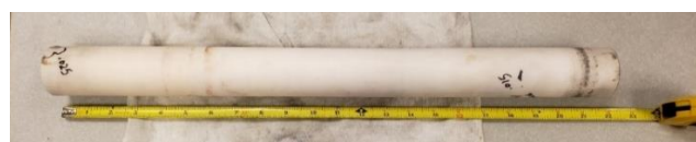
(b) Alumina process tube, 22.5 inches long with a 1.5 inch flange giving a 24 inch effective tube length.
