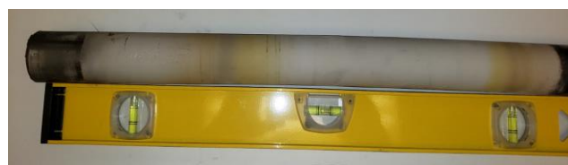
(a) Mullite tube after use showing bending.
