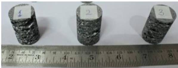
Fig. 1. 3 circular samples of 40mm were cut over EDM machine.
