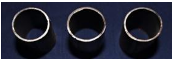
Fig. 2. 3 hollow tubes of 40mm height were cut using slow speed cutter.
