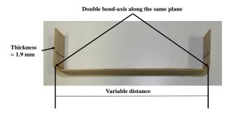
Fig. 1. The plywood sample used for the experiments.
