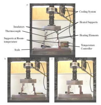
**Fig. 2.** Representation of a) the experimental setup, b) the rig during the experiment and c) the rig when the supports have reached the final position before retraction.
