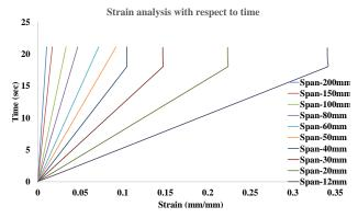
Fig. 3. Variations in the strains experienced due to changing the span lengths of the plywood from 200 mm to 12 mm.
