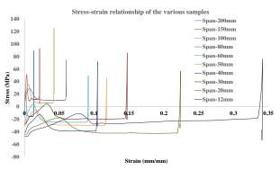
Fig. 5. Stress-strain analysis of the carious span lengths of the plywood from 200 mm to 12 mm.
