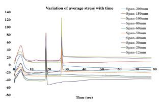
Fig. 4. Variations in the stresses experienced due to changing the span lengths of the plywood from 200 mm to 12 mm.
