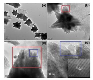
**Fig. 3.** HRTEM images of (a) large area TEM image, (b) TEM image of a single ZnO flower, (c) & (d) HRTEM images of the tip marked with red square and a blue square [inset of (d): lattice of ZnO flower] flower-shaped ZnO.
