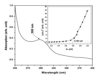
Fig. 5. UV-vis spectrum of flower-shaped ZnO (Inset: plot to determine direct band gap).
