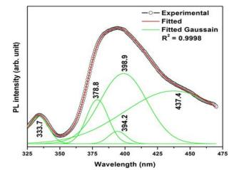
Fig. 6. Room temperature PL spectrum of flower-shaped ZnO (The Gaussian peaks marked in green colour at the bottom of the fitted curve which is marked in red colour).
