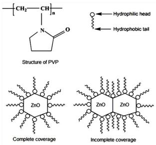
Fig. 4. Amphiphilic structure of PVP.
