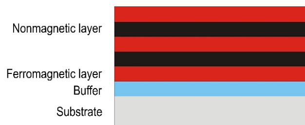
Fig. 9. Basic structure of a giant magnetoresistive device.
