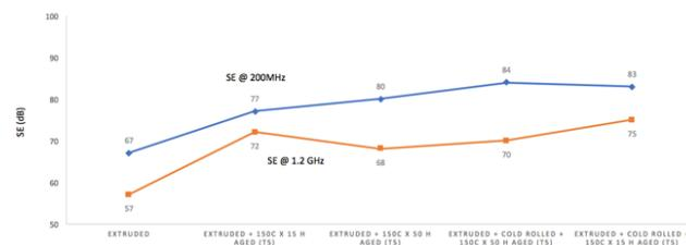
Fig. 5. EMI SE of ZK60 alloy at various testing frequency.
