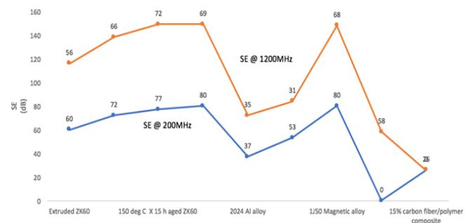
Fig. 2. Comparison of SE results among the ZK60 alloy and other shielding candidate materials.
