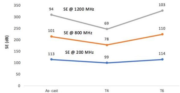
Fig. 1. EMI SE of Mg-4Zn alloy at varying testing frequencies for different heat treatment conditions.
