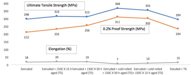
Fig. 4. Comparison of tensile properties of ZK60 alloys in different heat treatment states.
