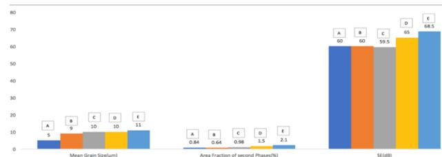
**Fig. 3.** Mean Grain Size, Area Fraction of Secondary Phases, SE comparison of ZK60 in various conditions (A= As Extruded, B = Solutionized, C = Solutionized and aged at 130deg C for 4h, D = Solutionized and aged at 130deg C for 20h, E = Solutionized and aged at 170deg C for 25h).
