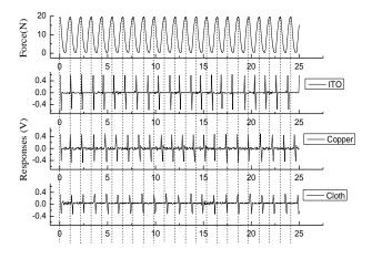
Fig. 7. Responses time of different sensor prototypes to periodic pressures.
