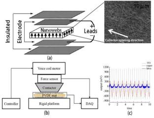
Fig. 1. Packaging structure of the PVDF nanofibers web as sensor prototype.
