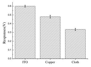
Fig. 4. The average responses of five sensor prototypes under the dynamic pressure loading (20N, 1Hz).
