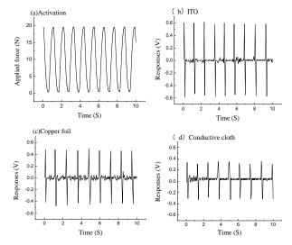
Fig. 3. Piezoelectric responses of different sensor prototypes to periodic compression forces.
