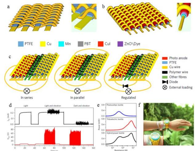
**Fig. 5.** T-ENG for both solar and mechanical energy harvesting. (a, b) Schematic structure of t-ENG and photovoltaic textile. (c) Solar cells and t-ENG electrical connected in series. (d) Short-circuit current and open-circuit voltage of the hybridizing system under the stimulation of light, vibration and light + vibration. Reproduced with permission [50]. Copyright © 2016, Rights Managed by Nature Publishing Group.
