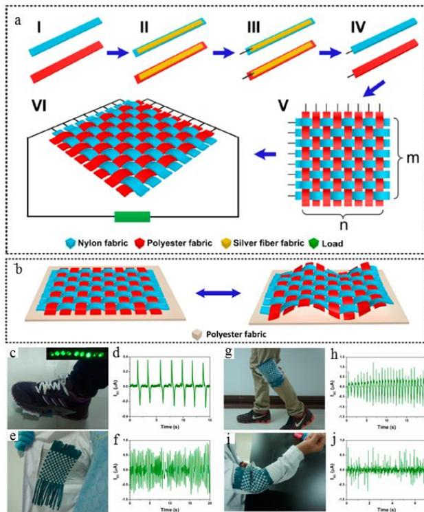
**Fig. 3.** T-ENG based on woven structure. (a, b) Schematic of TENG fabrication process. (c-j) TENG integrated to shoes, coats, and trousers to harvest different kinds of mechanical energy from body movements. Reprinted with permission from [33]. Copyright 2014 American Chemical Society.
