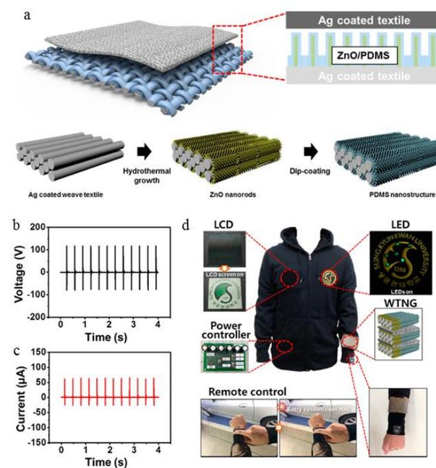
**Fig. 2.** A dominant design of t-TENG taking the advantage of rich surface morphologies. (a) Schematic of TENG fabrication process. (b, c) Output voltage and output current produced by t-TENG under a compressive force. (d) Different demonstrations of self-powered system by using the multilayer-stacked t-TENG. Reprinted with permission from [38]. Copyright 2015 American Chemical Society.
