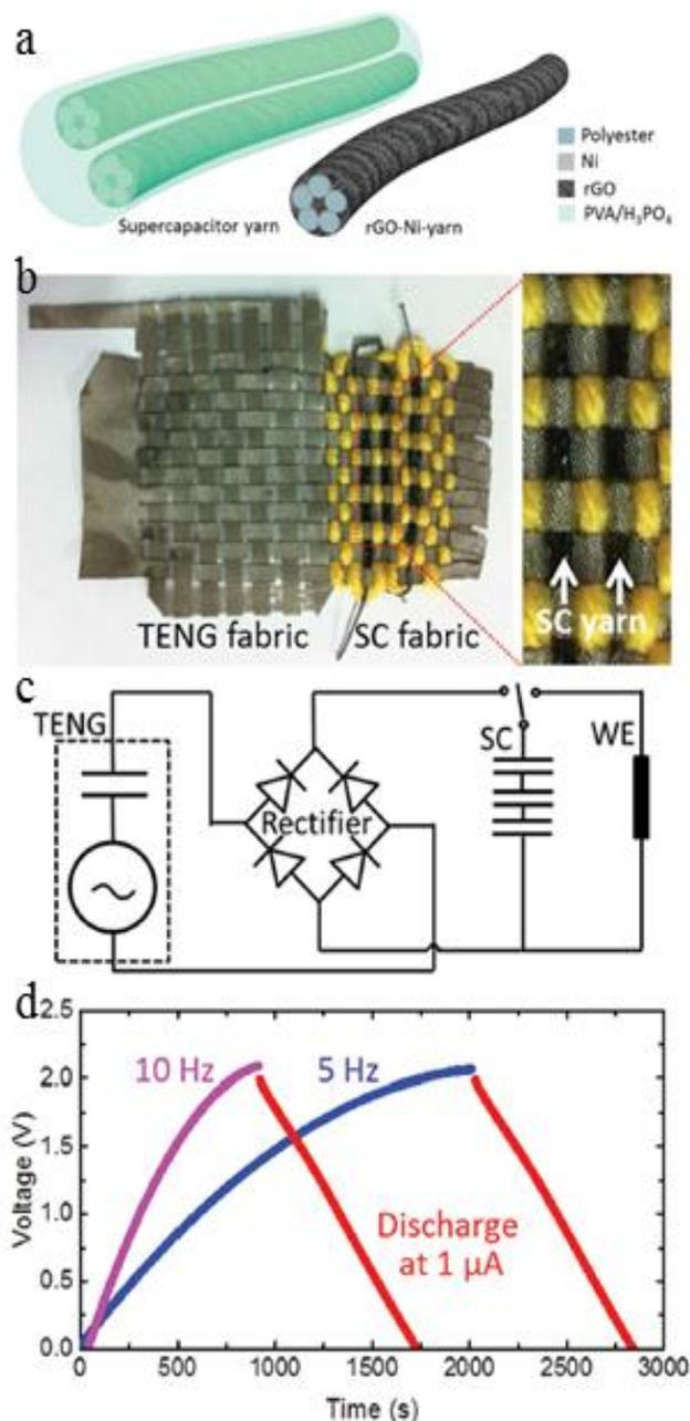
**Fig. 6.** Textile based super capacitor and lithium-ion battery integrated with t-TENG. (a) Schematic structure of yarn supercapacitor. (b) Yarn supercapacitors in series connection integrated with a t-TENG fabric. (c) The equivalent circuit of the self-charging power textile. (d) Voltage profile of the supercapacitors. Reproduced with permission [44]. Copyright 2016, WILEY-VCH Verlag GmbH & Co. KGaA, Weinheim.
