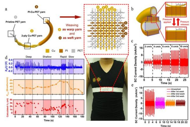
**Fig. 4.** An energy harvesting fabric by loom weaving. (a, b) Schematic of TENG fabrication process and working principle. (c) Short-circuit current of the t-ENG when fabric is tapped. (d) Respiration monitoring realized by integrated the fabric into a chest strap. (e) A remarkable washing durability. Reproduced with permission [49]. Copyright 2016, WILEY-VCH Verlag GmbH & Co. KGaA, Weinheim.
