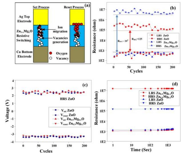
**Fig. 4.** (a) Schematic diagram of the switching mechanism of  $\text{Ag}/\text{Zn}_{1-x}\text{Mg}_x\text{O}/\text{Cu}$  memory cell, (b) Endurance performance of  $\text{Ag}/\text{Zn}_{1-x}\text{Mg}_x\text{O}/\text{Cu}$  thin films for 200 switching cycles at 1V read pulse, (c) Set and reset voltage distribution of both films and (d) Data retention property of both memory cells.
