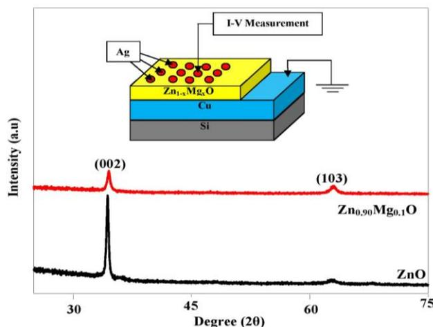
**Fig. 1** X-ray diffraction pattern of ZnO and  $Zn_{0.9}Mg_{0.1}O$  films. The inset shows schematic structure of the  $Ag/Zn_{1-x}Mg_xO/Cu$  ReRAM memory cell.
