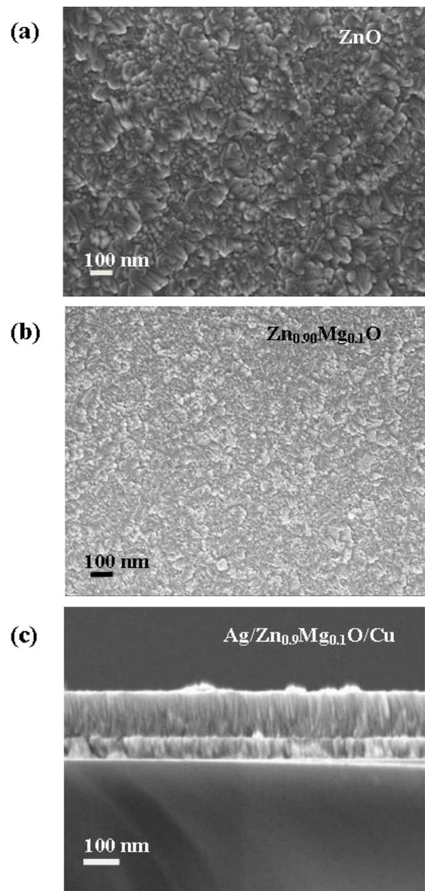
**Fig. 2** (a), (b) shows FE-SEM image of ZnO and  $Zn_{0.9}Mg_{0.1}O$  thin films respectively and (c) Cross sectional FE-SEM image of  $Zn_{0.9}Mg_{0.1}O/Cu/Si$  film.
