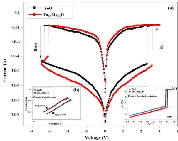
**Fig. 3** (a) Typical bipolar resistive switching characteristics for Ag/Zn<sub>1-x</sub>Mg<sub>x</sub>O/Cu memory cell for a DC voltage sweep (0V→3.5V→0V→-3.5V→0V). Conduction mechanism of Ag/Zn<sub>1-x</sub>Mg<sub>x</sub>O/Cu thin film (b) Ohmic conduction in LRS region and (c) Poole-Frenkel emission in HRS region.
