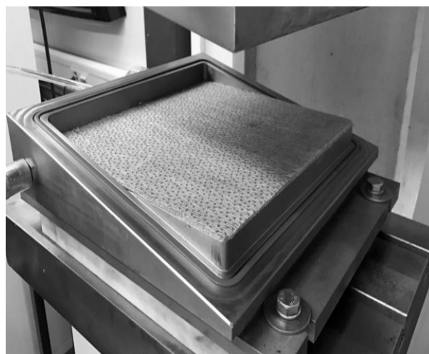
Fig. 3. RTM processing using plate tool; dry flax fiber preform placed on lower die (mounted on press)
