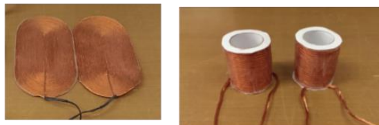
The magnetic coil configuration, (a) pancake coil, (b) classic cylindrical Coilrack deflection
