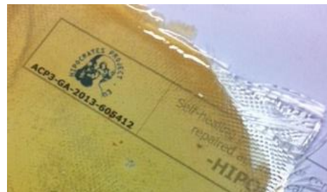
Fig. 6. Glass fiber reinforced Diels-Alder functionalised epoxy composite after fabrication.
