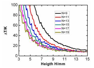
**Fig. 4.** The influence of filament height (*H*) on  $\Delta Ty$  at difference filament numbers when filament length *L* is 160 mm.
