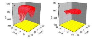
Fig. 8. The temperature field distribution of 100-mm substrate at equal-space (a) and unequal-space filament arrays (b). Filament array parameters are chosen as L=160 mm, H=11.5 mm, N=11. Here, "X" stands for the direction parallel to filaments, and "Y" stands for the direction perpendicular to filaments.
