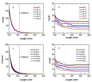
and edge along X axis and (b) Y axis at H=9.4 mm. (c) The temperature difference between center and edge along X axis and (d) Y axis at N=15.
