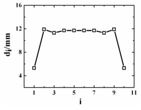
**Fig. 7.** The space distribution between each two adjacent filaments when *L* is 160 mm H is 11.5 mm and *N* is 11.
