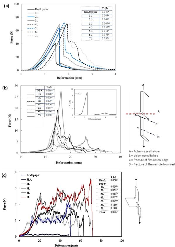
**Fig. 3.** Mechanical patterns of uncoated and PLA coated Kraft paper: (a) typical curves of puncture resistance; (b) heat-sealing resistance and the associated failure modes; (c) tear-propagation resistance profile. The number of the layers (L) is indicated in the legend. Table inset shows the tenacity (T) values for each assay.
