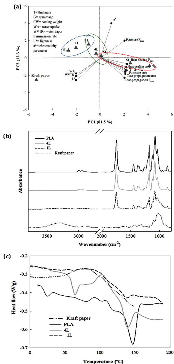
**Fig. 4.** (a) PCA biplots summarize the relationships between Kraft paper samples impregnated with different layers of PLA, and physicochemical, optical, and mechanical properties. Spectroscopic and thermal studies of Kraft paper coated with different layers of PLA by means of: (b) ATR-FTIR, (c) DSC.
