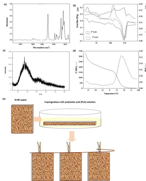
**Fig. 1.** Spectroscopic and thermal studies of PLA films by mean of: (a) ATR-FTIR, (b) DSC, (c) X-ray and (d) DMA techniques. Representative scheme of the steps involved in the preparation of the PLA coated Kraft Paper (e).
