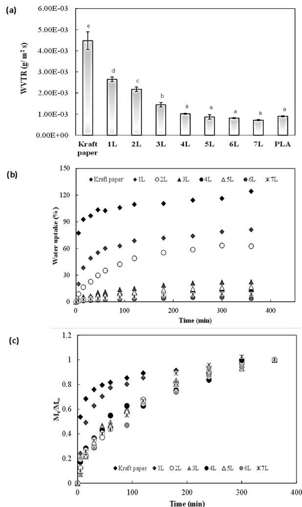
**Fig. 2.** (a) Water vapor transmission rate (WVTR) of uncoated and coated Kraft paper with different layers of PLA; (b) percentage of water uptake (WA) of uncoated and coated Kraft paper with different layers of PLA; (c) fraction of water uptake ( $M_t/M_\infty$ ). The values correspond to the arithmetic average of three measurements.
