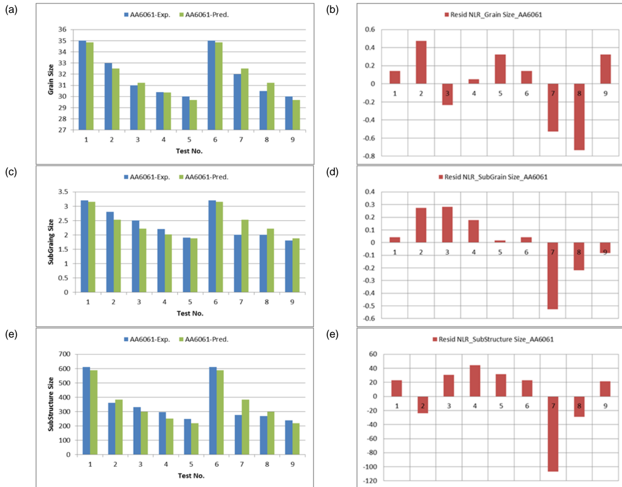
Fig. V. Experimental results vs. predicted (a, c, and e) and theresiduals distribution (b, d, and f) for (a, b) grains size, (c, d) sub-grains size, and (e, f) substructure size.
