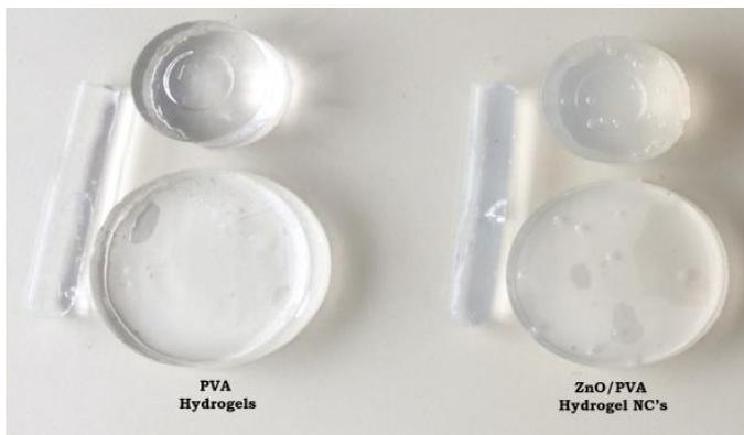
**Fig.** PVA and ZnO/PVA hydrogel nanocomposites.
