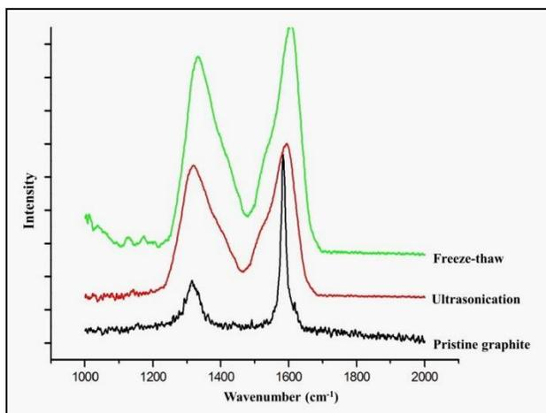
**Fig. 4.** Raman spectrum of exfoliated graphene oxide by Freeze-thaw technique in comparison with ultrasonication technique and pristine graphite.
