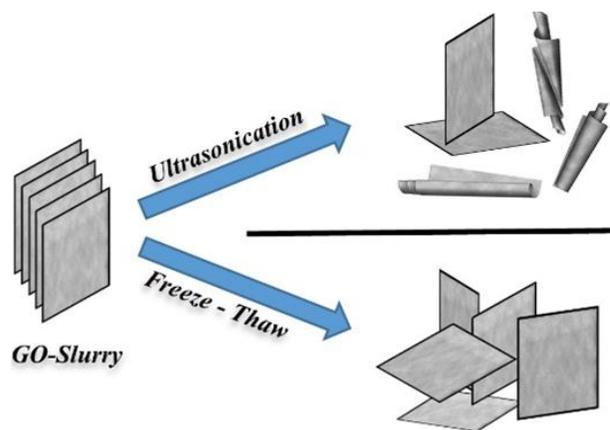
Fig. 1. Exfoliation of graphitic planes by freezing and thawing and ultrasonication.
