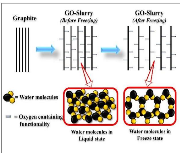
Fig. 2. Mechanism of exfoliation during freeze-thaw cycles.
