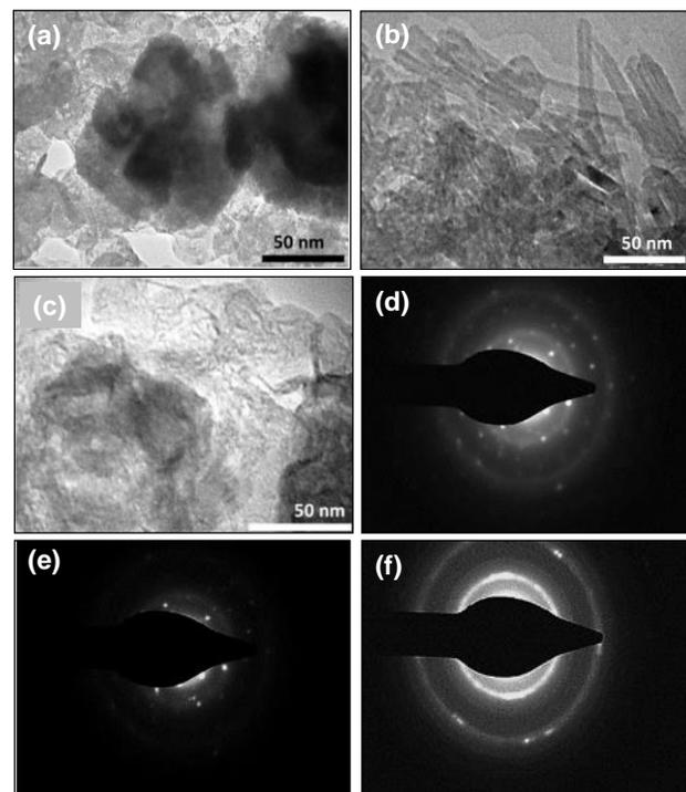
Fig. 3. TEM images of (a) GO-slurry, (b) exfoliated graphitic planes and scrolls by ultrasonication, (c) exfoliated graphitic planes by freezing and thawing, and SAED images of (d) GO slurry, (e) exfoliated graphitic planes and scrolls by ultrasonication, and (f) exfoliated graphitic planes by freezing and thawing.
