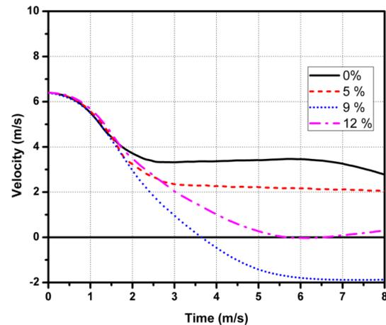
Fig. 6. Velocity-time response of nanocomposites subjected to 110 J.
