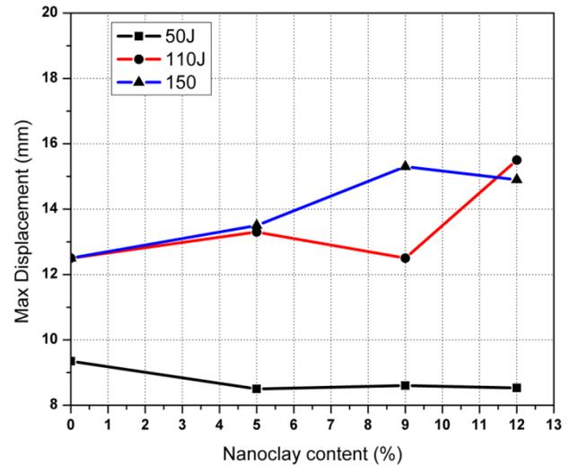
Fig. 5. Maximum displacement - nanoclay content under different impact energies.
