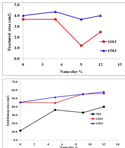
**Fig. 8.** Effect of Nano clay on fractured area and damage area of the laminates.
