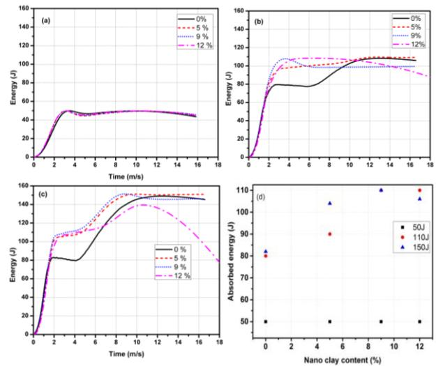
**Fig. 3.** Energy-time response at (a) 50 J (b) 110 J (c) 150 J and (d) absorbed energy.
