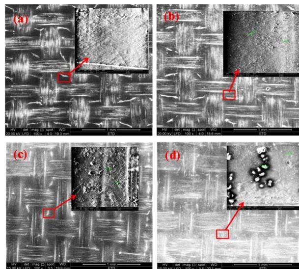
**Fig. 1.** SEM images of different nanoclay content composite laminates (a) 0% (b) 5% (c) 9% (d) 12%.
