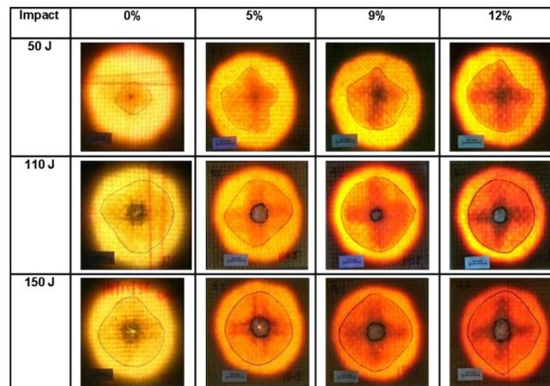
**Fig. 7.** Backlit images of different nanocomposite laminates subjected to different impact energy.
