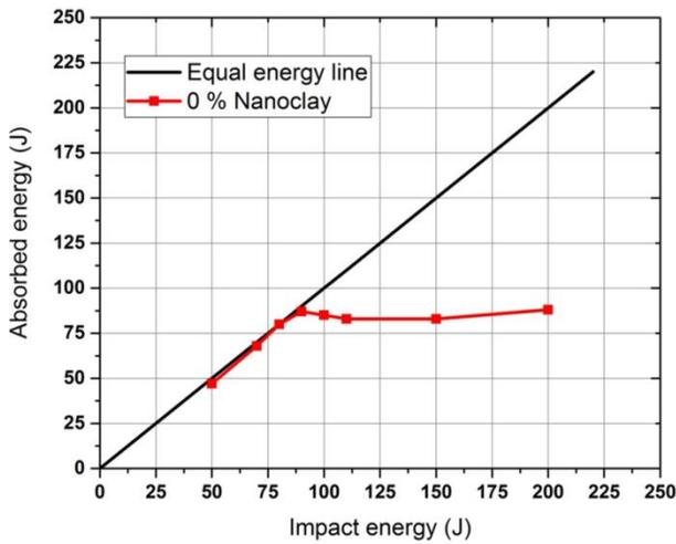
**Fig. 2.** Energy profile diagram for pristine laminate.
