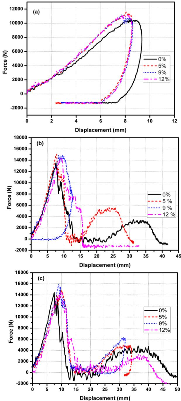
Fig. 4. Force Vs displacement for laminates impacted at (a) 50J (b) 110J (c) 150J.
