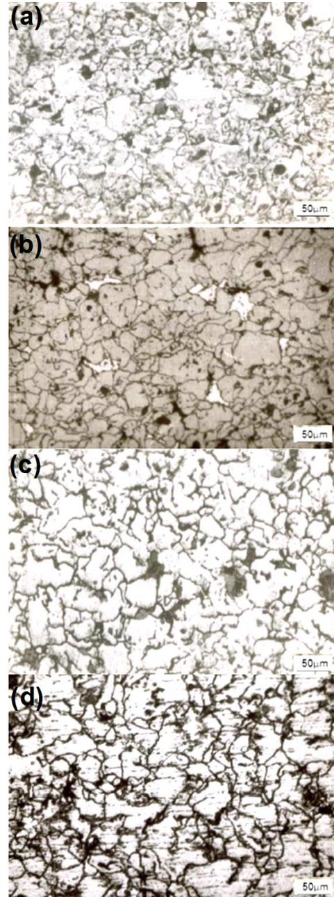
**Fig. 2.** Microstructure of Fe-5Cu-xPb alloys hot pressed at a pressure of 300 MPa and a temperature of 500 °C for 10 min for a Pb percentage of (a) 0, (b) 4, (c) 8, (d) 12 wt%.
