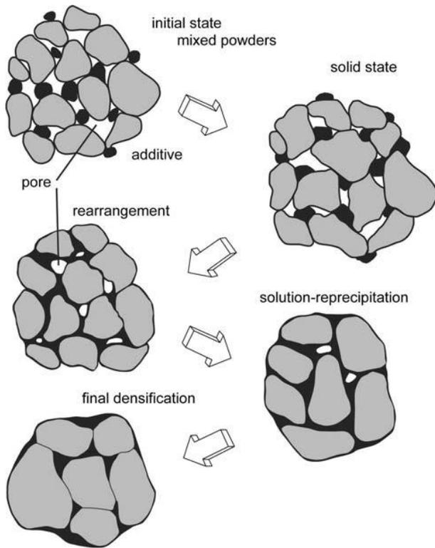
Fig. I. A schematic of the microstructure changes during LPS [16].
