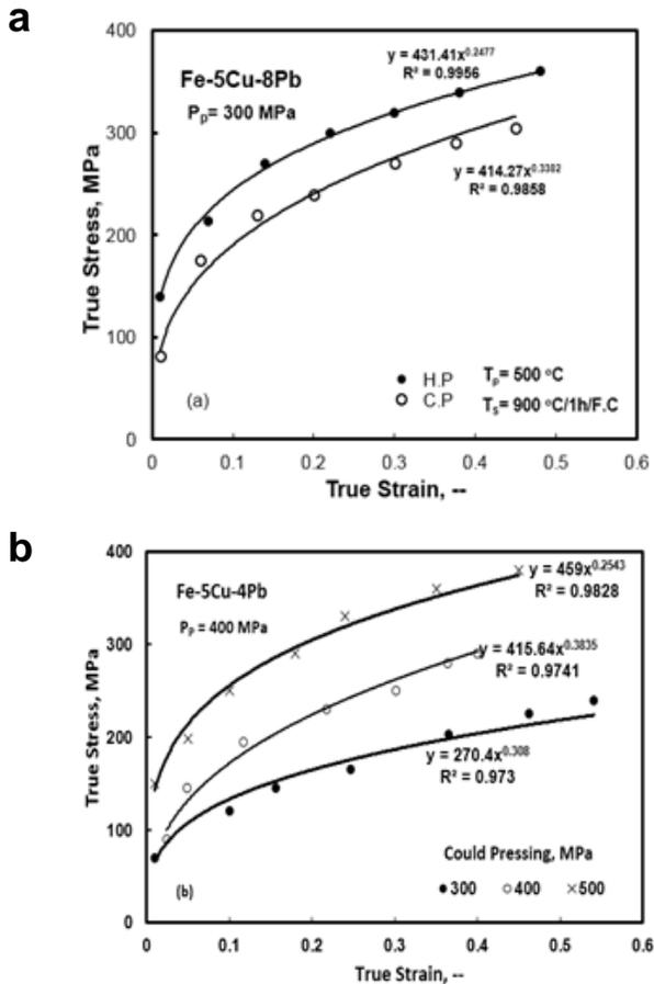
**Fig. 6.** True stress-strain curves for (a) Fe-5Cu-8Pb and (b) Fe-5Cu-4Pb alloys processed using (a) hot and cold compaction and (b) cold compacted at 300, 400, and 500 MPa.
