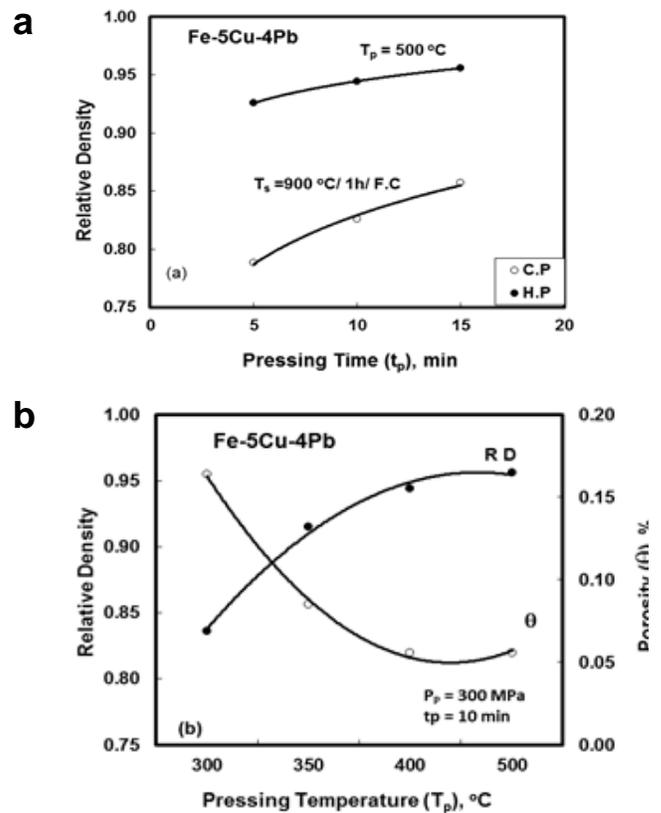
Fig. IV. The effect of (a) compaction time and (b) compaction temperature on (a, b) the relative density and (b) porosity of Fe-3Cu-5Pb alloy.
