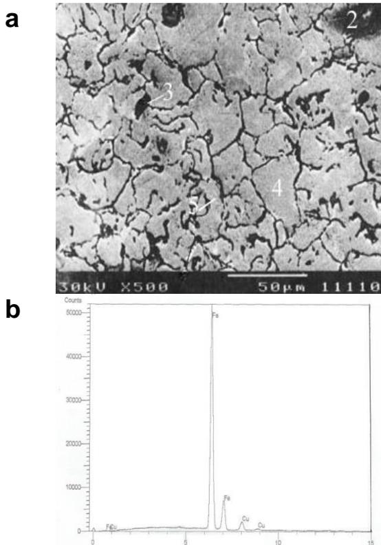
**Fig. 4.** (a) SEM and (b) spot locations (of point 2 in Fig. 4a) of EDX analysis for Fe-5Cu-8Pb hot pressed alloy at 300 MPa/500 °C/10 min.
