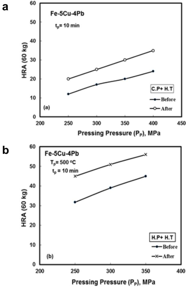
Fig. V. Effect of heat treatment on hardness values of (a) cold and (b) hot compaction Fe-5Cu-4Pb alloy.
