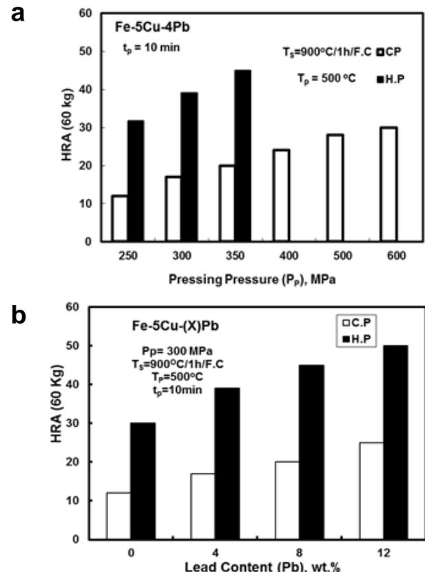
**Fig. 7.** The effect of (a) compaction pressure on the hardness of Fe-5Cu-4Pb alloy and (b) Pb content on the hardness of Fe-5Cu-(x)Pb alloys.
