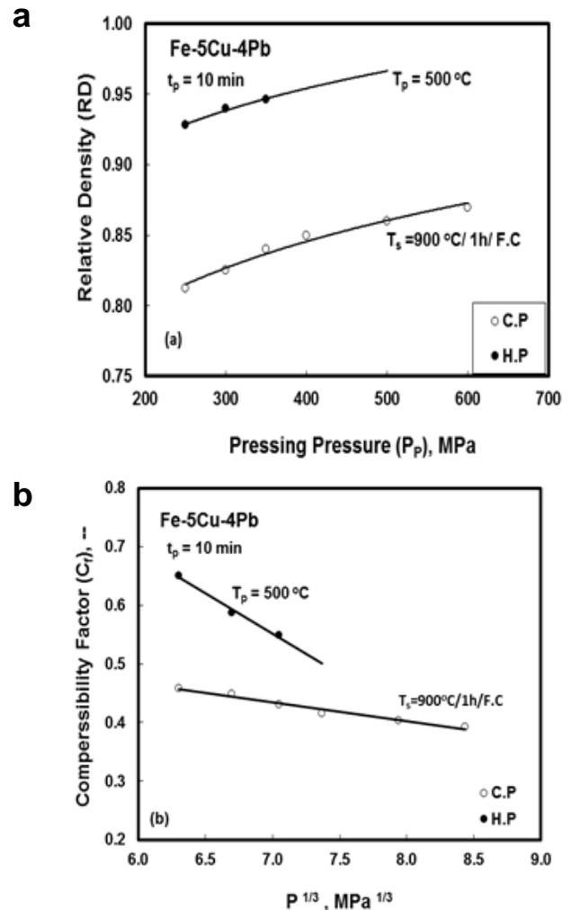
**Fig. 5.** The influence of the compaction pressure on (a) the relative density and (b) the compressibility factor of cold and hot compacted Fe-5Cu-4Pb compacts.
