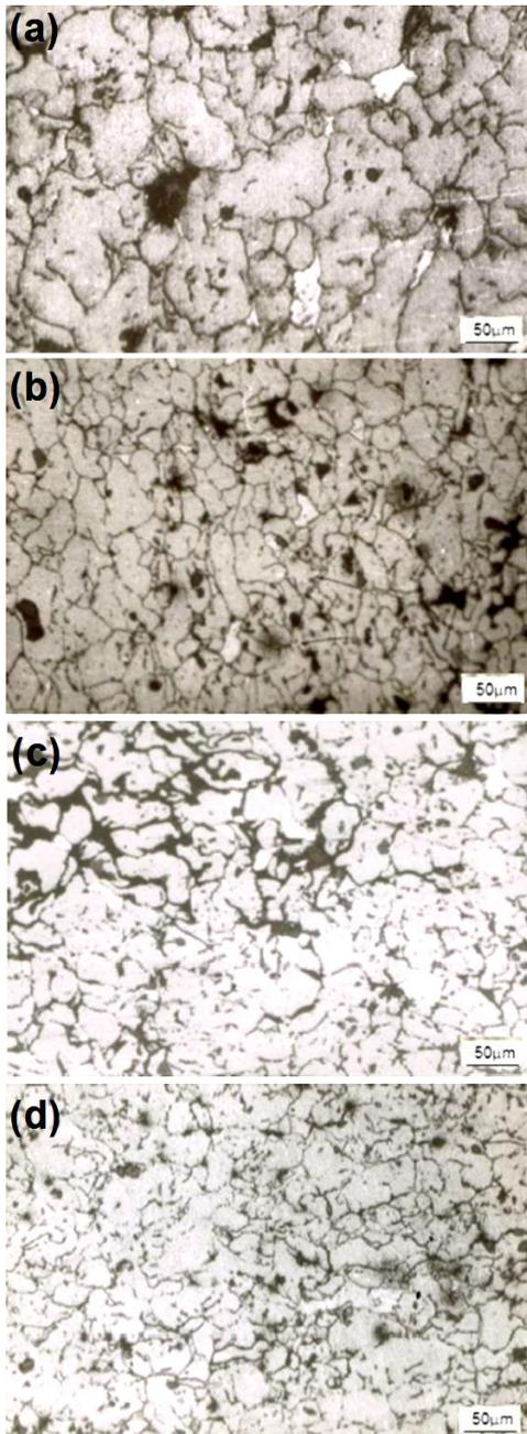
**Fig. 3.** Microstructure of (a, c) cold pressed and (b, d) hot pressed Fe-5Cu-4Pb alloy pressed at a pressure of (a, b) 250 MPa and (c, d) 350 MPa.
