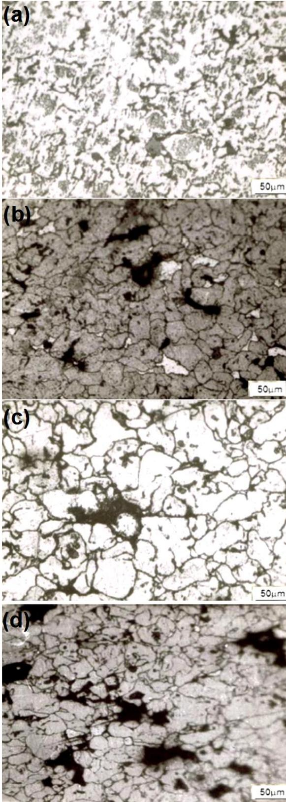
**Fig. 1.** Microstructure of Fe-5Cu-xPb alloys cold pressed at 300 MPa for 10 min and sintered at 900°C/1 h/FC for a Pb percentage of (a) 0, (b) 4, (c) 8, (d) 12 wt%.
