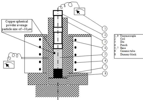
Fig. II. Die setup of the hot compaction powder metallurgy compaction technique.
