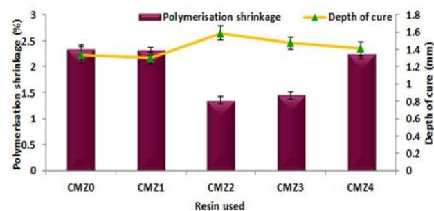
**Fig. 3.** Polymerisation shrinkage and depth of cure of composites prepared from from IOHRs containing mixture of alkoxides of calcium/magnesium/zinc: effect of variation of calcium content from 0 to 0.3%.
