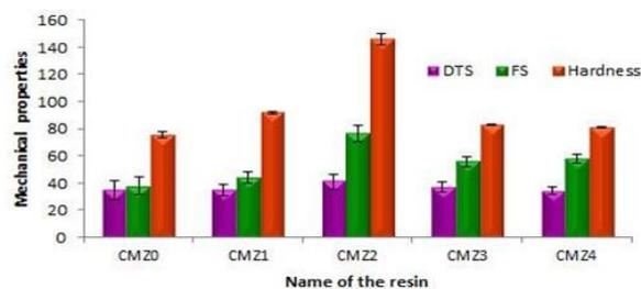
**Fig. 2.** DTS, FS and hardness of VLCs prepared from IOHRs containing mixture of alkoxides of calcium/magnesium/zinc: effect of variation of calcium content from 0 to 0.3%.
