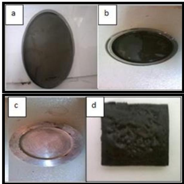
**Fig. 1.** Actual photographs of the samples (a) Thin film of Ag/PPy-PVA prepared in a glass petridish (b) Thin film prepared in a mould (c) Mould used for preparation of thin film (d) Thick film of Ag/PPy-PVA nanocomposites.
