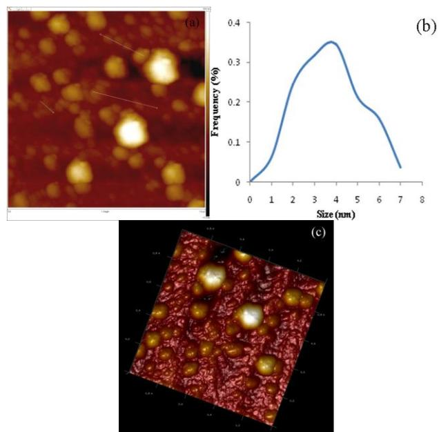
Fig. 5. (a) AFM images of synthesized AgNPs in 2D form, (b) Particles size distribution and (c) 3D form of particles.
