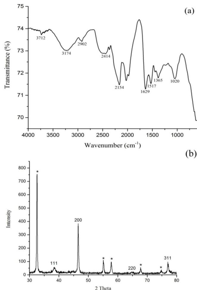
**Fig. 2.** (a) FTIR spectrum of synthesized AgNPs and (b) XRD pattern of synthesized AgNPs, asterisks indicate unassigned peaks may be due to the present of proteins in culture supernatant.
