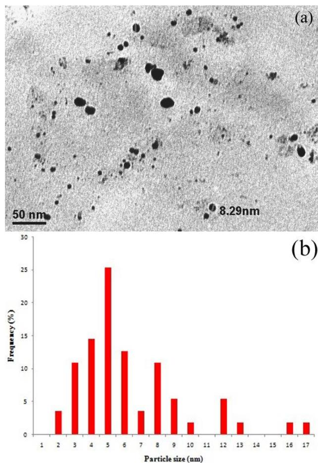
Fig. 3. (a) HR-TEM micrograph of synthesized AgNPs and (b) Particles size histogram.
