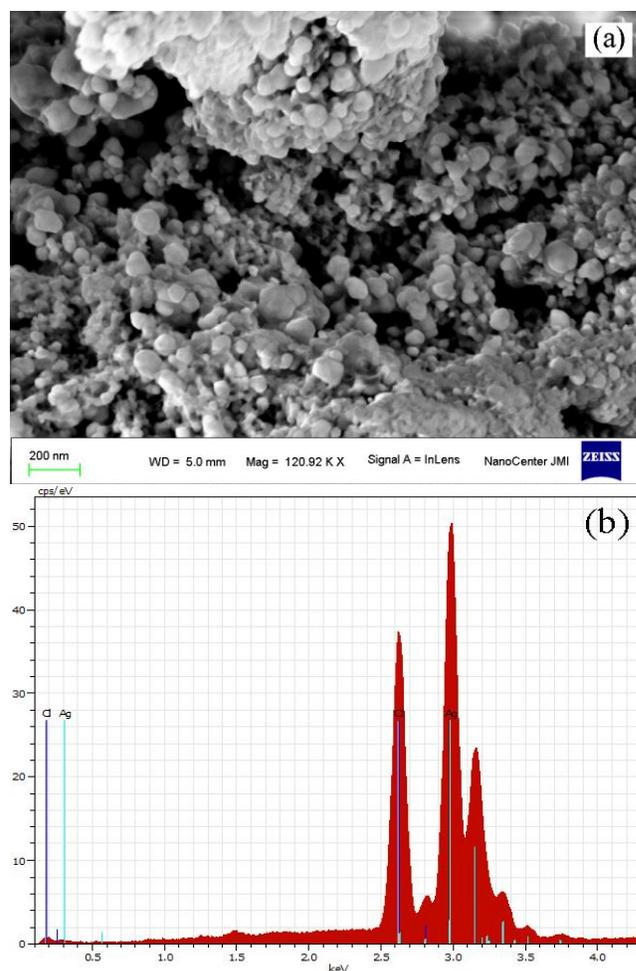
Fig. 4. (a) FE-SEM micrograph and (b) EDX spectrum of synthesized AgNPs.
