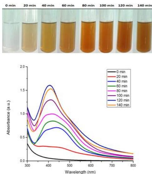
**Fig. 1.** UV-vis spectra of AgNPs synthesized at different time intervals.
