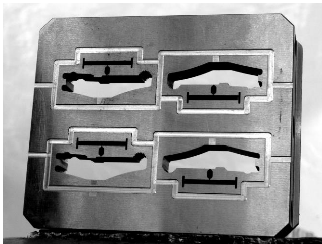
Fig. 8. Die plate for injection plastic mould produced from stainless steel 12X18H10T (AISI 321).
