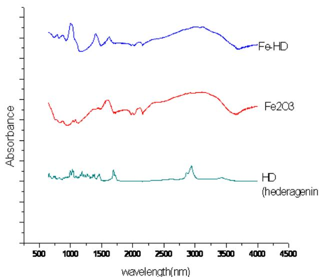
**Fig. 3.** FT-IR spectra of magnetic nanoparticles, pure hederagenin (HD), and hederagenin-coated magnetic nanoparticles (HMPs).
