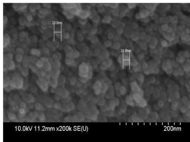
**Fig. 1.** Scanning electron micrograph image of Hederagenin-coated magnetic nanoparticles (HMPs).
