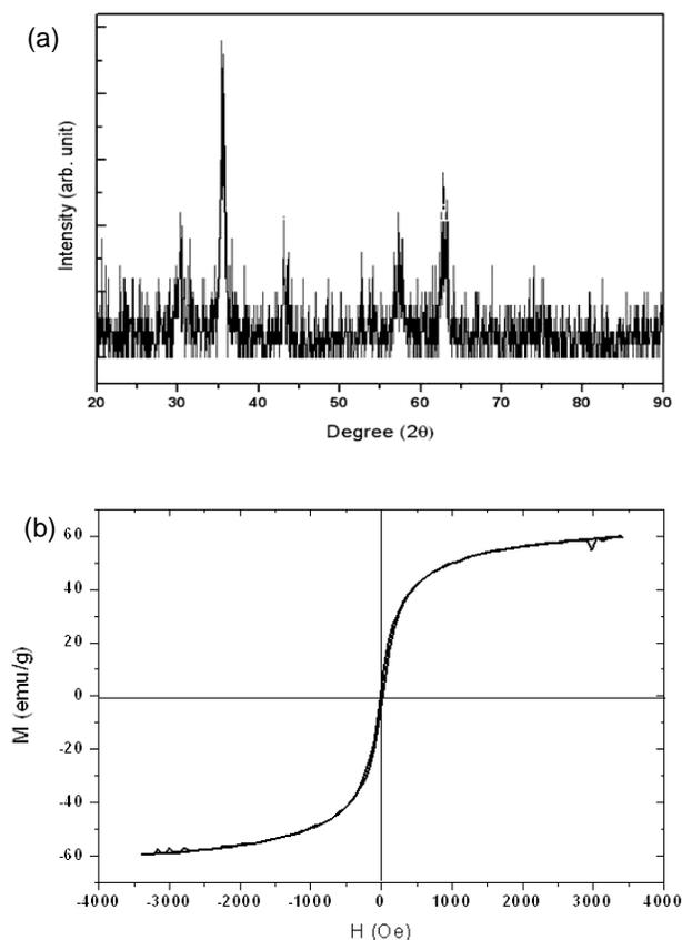
**Fig. 2.** XRD patterns (a) and vibrating sample magnetometer (b) of Hederagenin-coated magnetic nanoparticles (HMPs).
