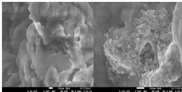
**Fig. 3.** SEM of native tea leaves (left) and tea leaves modified by direct ferrofluid treatment (right). Reproduced, with permission, from [14].
