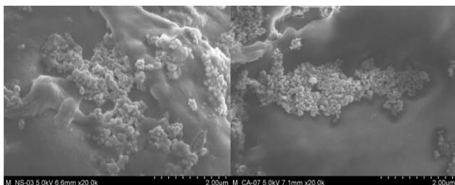
**Fig. 5.** SEM image of native (left) and chemically treated (right) barley straw magnetically modified with microwave synthesized magnetic iron oxides nano- and microparticles. Reproduced, with permission, from [18].
