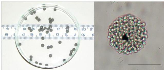
**Fig. 10.** Magnetically responsive alginate beads containing entrapped *Saccharomyces cerevisiae* cells and magnetite microparticles. Millimeter-sized beads (left) and microbeads (right; the scale bar corresponds to 50 µm). Reproduced, with permission, from [39].
