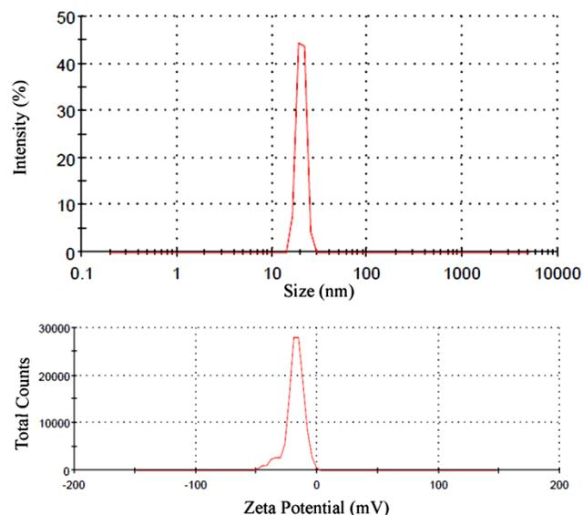
Fig. S4. Particle size and zeta potential distribution plots of biosynthesized AgNPs.
