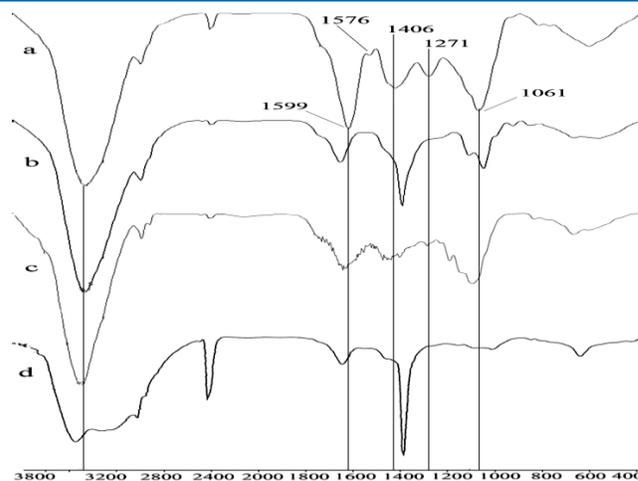
**Fig. 6.** FTIR spectra of (a) untreated leaf extract, (b) treated leaf extract, (c) AgNPs and (d) silver nitrate.
