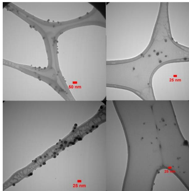
**Fig. 4.** TEM micrographs of silver nanoparticles.
