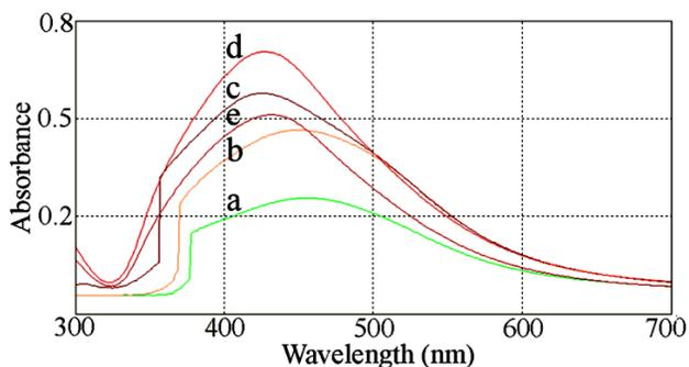
**Fig. 1.** The UV-vis spectra of AgNPs prepared in different amounts of leaf extract, a: 10, b: 5, c: 2.5, d: 1 and e: 0.5 mL leaf extract.
