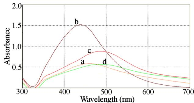
**Fig. 3.** The UV-vis spectra of AgNPs synthesised in different temperatures, a: 15°C, b: 28°C, c: 50°C and d: 70°C.
