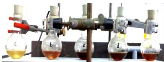
Fig. S2. A brown-yellow colour appearance after 1.5h reaction at various leaves extract quantities, a: 10, b: 5, c: 2.5, d: 1 and e: 0.5 mL leaf extract in a 10 mL reaction containing AgNO<sub>3</sub> (1mM).
