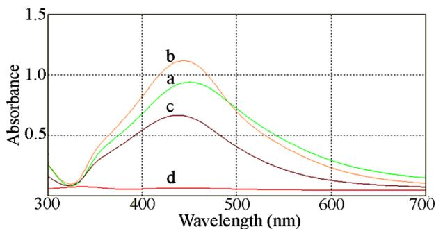
**Fig. 2.** The UV-vis spectra of AgNPs prepared in different concentrations of  $\text{AgNO}_3$ , a: 10, b: 5, c: 1 and d: 0.1 mM.
