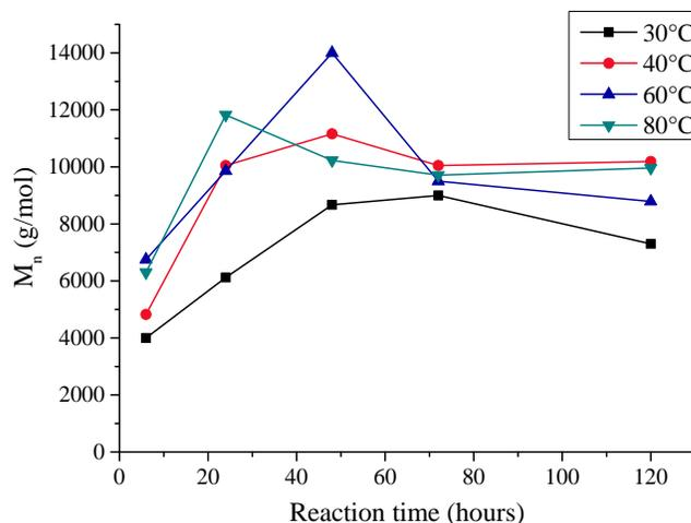
**Fig. 1.** Effect of temperature on  $M_n$  of PCL samples.
