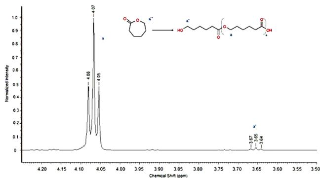
**Fig. 3.** <sup>1</sup>H NMR spectrum of polymer sample.
