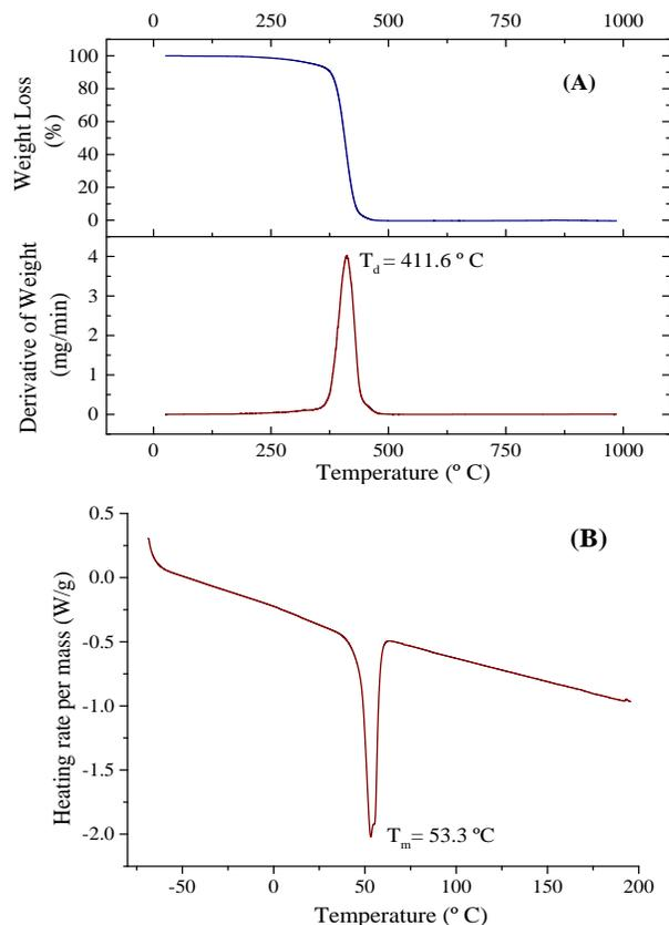
**Fig. 4.** TGA (A) and DSC (B) curves of polymer sample.
