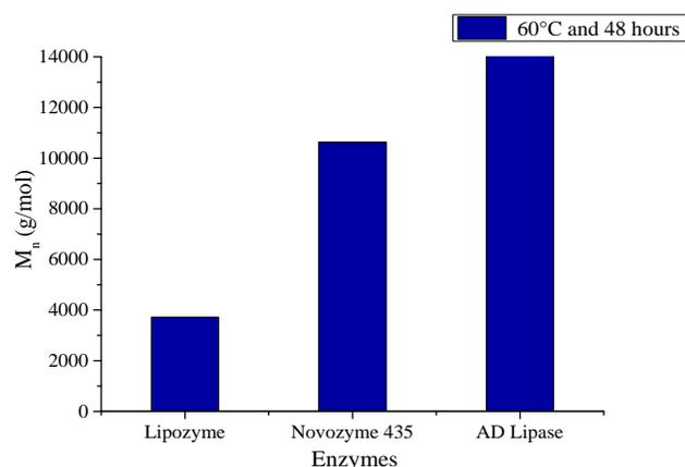
**Fig. 6.** Molecular weights of polymer samples obtained via commercial lipases and new immobilized CALB.
