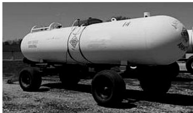
Fig. 1. Anhydrous ammonia nurse tank on running gear. (Photo courtesy of the U.S. Federal Motor Carrier Safety Administration).
