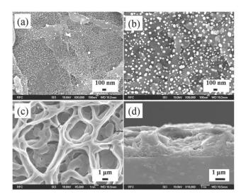
**Fig. 5.** Field emission scanning electron micrographs(FESEM) of (a) Au-TiO<sub>2</sub> spray coated at the 100 nm scale, (b) Au-TiO<sub>2</sub> spray coated and annealed samples at the 100 nm scale, (c) TiO<sub>2</sub> spray coated at 400°C at the 1  $\mu$ m scale and (d) crosssectional micrographs of TiO<sub>2</sub> spray coated at 400°C at the 1  $\mu$ m scale.
