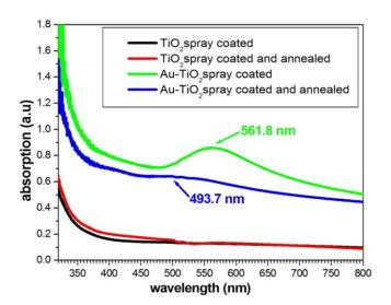
**Fig. 3.** Ultra violet-visible (UV-Vis) absorption spectra of the  $TiO_2$  spray coated;  $TiO_2$  spray coated and annealed; Au-TiO\_2 spray coated; Au-TiO\_2 spray coated and annealed samples.
