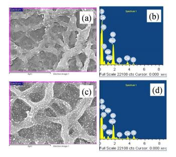
**Fig. 6.** (a) FESEM micrograph area selected for EDX pattern of Au-TiO<sub>2</sub> spray coated film; (b) EDX pattern of Au-TiO<sub>2</sub> spray coated film; (c) FESEM micrograph area selected for EDX pattern of Au-TiO<sub>2</sub> spray coated annealed film; (d) EDX pattern of Au-TiO<sub>2</sub> spray coated annealed film.
