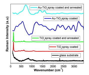
Fig. 2. Raman spectra of the glass substrate;  $TiO_2$  spray coated;  $TiO_2$  spray coated;  $TiO_2$  spray coated;  $Au-TiO_2$  spray coated;  $Au-TiO_2$  spray coated and annealed samples.
