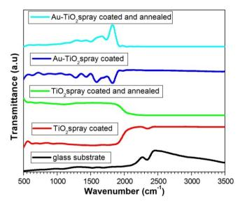
Fig. 4. FTIR spectra of the glass substrate;  $TiO_2$  spray coated;  $TiO_2$  spray coated and annealed; Au-TiO\_2 spray coated; Au-TiO\_2 spray coated and annealed samples.
