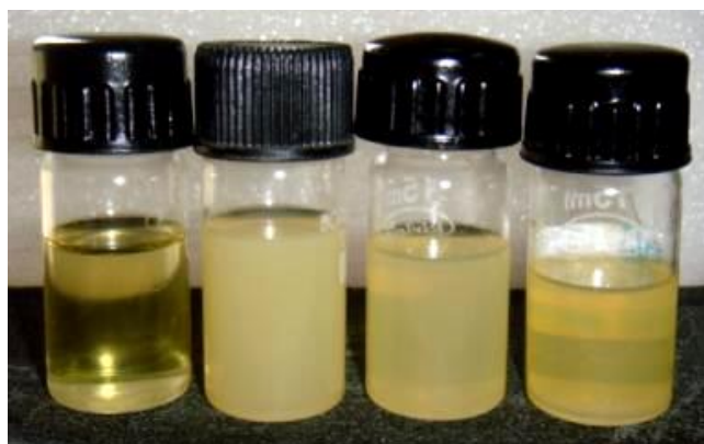
Fig 3. Photographic image of alumina nanofluids (a) pure biodiesel (b) 0.1 VF (c) 0.2 VF and (d) 0.5 VF after 30min of preparation.
