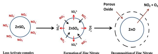
**Scheme 2.** Schematic representation of the decomposition of ZnSO<sub>4</sub> in NaNO<sub>3</sub>-KNO<sub>3</sub> eutectic mixture.
