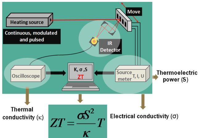
**Supporting Fig. 1.** Experimental micro ZT meter with simultaneous heating and measurement of voltage and temperature.
