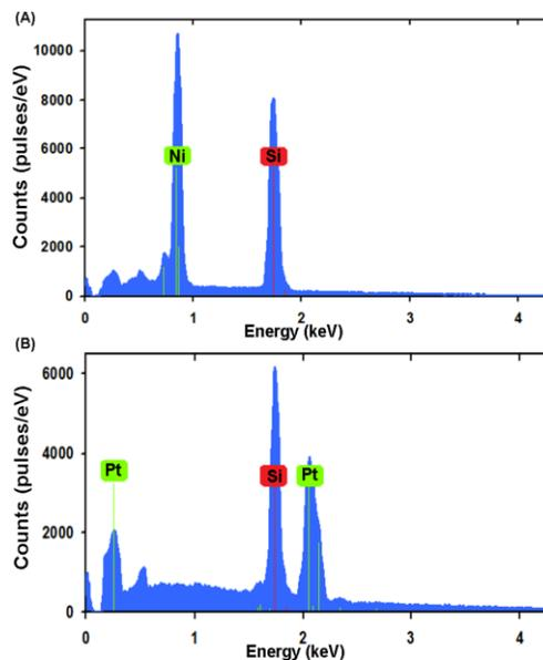
Fig. 4. EDX spectroscopy measured for the formed (A) NiSi film and (B) PtSi film.
