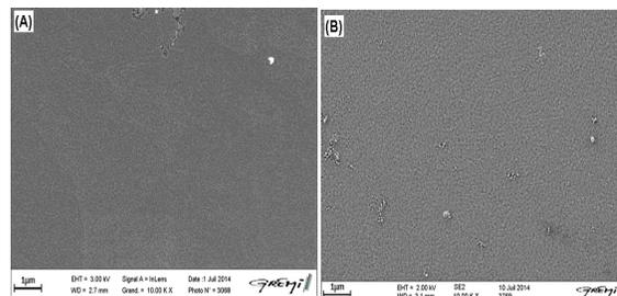
Fig. 5. Morphological investigation by SEM of the surface of the formed (A) Ni-silicide and (B) Pt-silicide.
