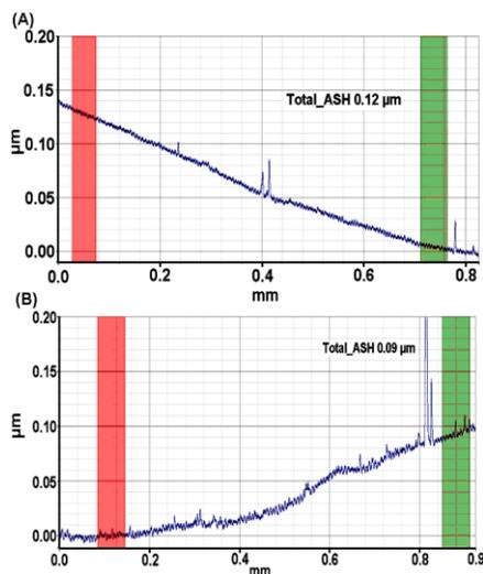
Fig. 3. Profilometer analysis of the formed (A) NiSi film and (B) PtSi film.
