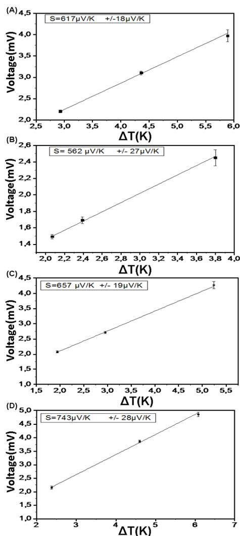
Fig. 6. Thermoelectric investigation of the four samples prepared: (A) Ni/Si, (B) Pt/Si, (C) NiSi/Si and (D) PtSi/Si.
