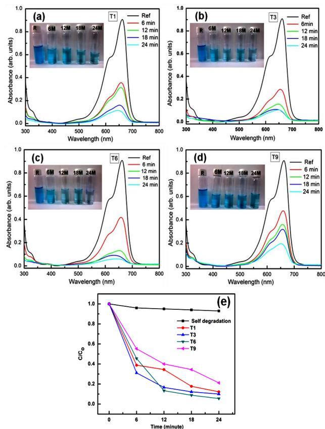
**Fig. 4.** (a-d) Optical absorption spectra showing temporal evolution of sun light driven photocatalytic degradation of MB in water using samples T1, T3, T6 and T9 as photocatalysts. (e) Kinetics of photocatalytic degradation of MB in water using samples T1, T3, T6 and T9 as photocatalysts.
