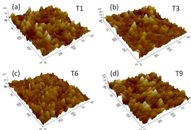
**Fig. 3.** (a-d) Three dimensional AFM images of  $\text{TiO}_2$  nanostructures in the samples T1, T3, T6 and T9.
