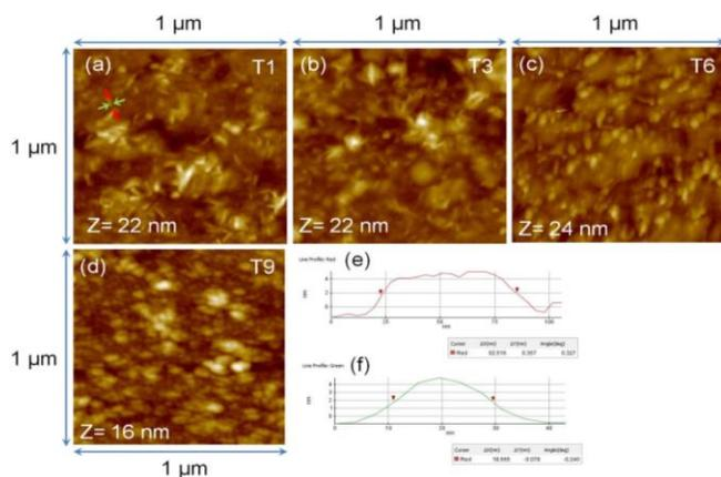
**Fig. 2.** (a-d) AFM images of  $\text{TiO}_2$  nanostructures in the samples T1, T3, T6 and T9, (e-f) line profiles across length and width of one nanorod marked in (a).
