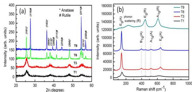
**Fig. 1.** (a) XRD patterns of nanostructured TiO<sub>2</sub> samples T1, T3, T6 and T9 and (b) Raman spectra of nanostructured TiO<sub>2</sub> samples T1, T3, T6 and T9.
