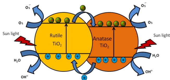
**Fig. 5.** Schematic diagram showing processes leading to sun light driven photocatalytic activity of TiO<sub>2</sub> nanostructures.
