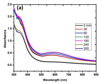
Fig. 1. UV-vis spectra of synthesized AuNPs.
