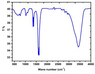
Fig. 2. FT-IR spectra of AuNPs.
