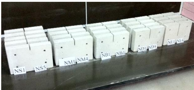
Fig. 2. Specimens after notching.
