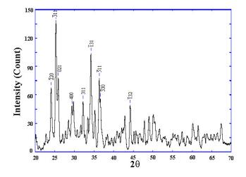
Fig. 1. X-ray diffraction pattern of  $SrAl_4O_7$ :Dy phosphor matched with JCPDS data file no. 25-1208.
