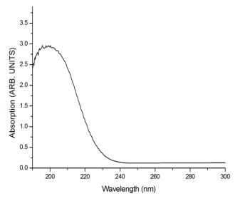
Fig. 2. Absorption spectra of SrAl<sub>4</sub>O<sub>7</sub>:Dy having absorption edge 242nm.
