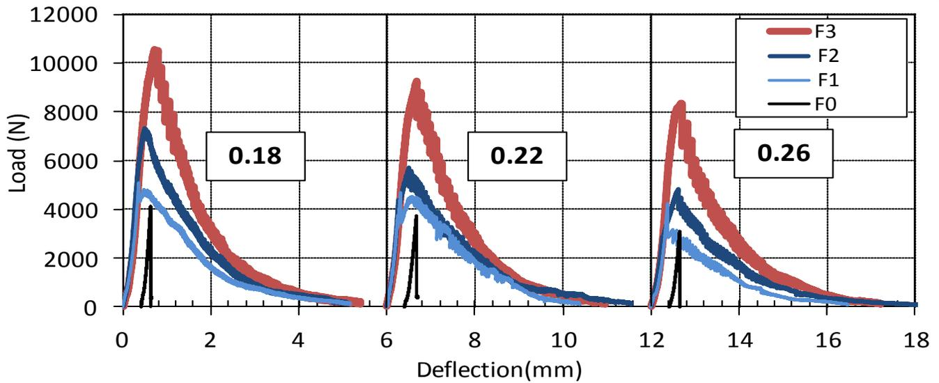
Fig. 4. Load vs. mid-span deflection curves of RPC specimens.
