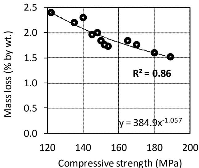
**Fig. 9.** Compressive strength vs mass loss.
