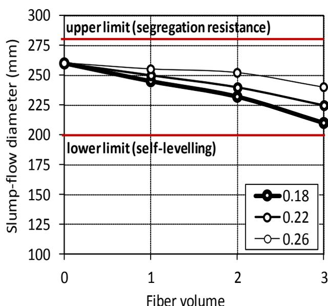
**Fig. 3.** Slump-flow diameter depending on W/C ratio and fiber volume.
