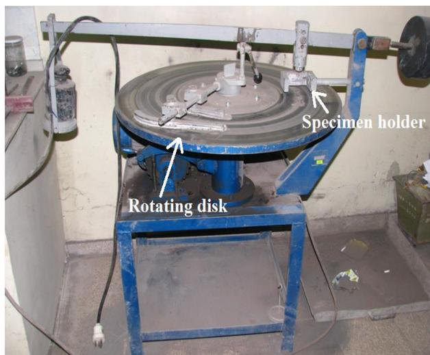
**Fig. 1.** Böhme apparatus used for abrasion test.
