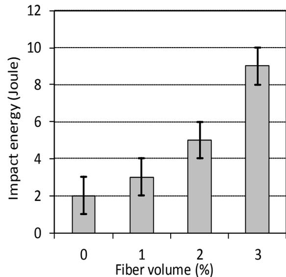
**Fig. 11.** Charpy impact test results.
