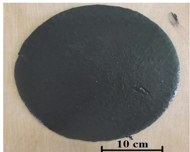
**Fig. 2.** The mini-slump flow testing of fresh RPC.
