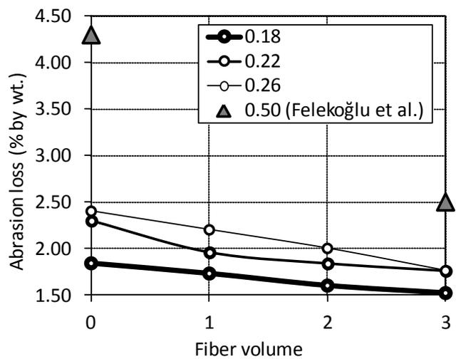
Fig. 8. Abrasion loss (% by wt.) depending on fiber volume and W/C ratio.
