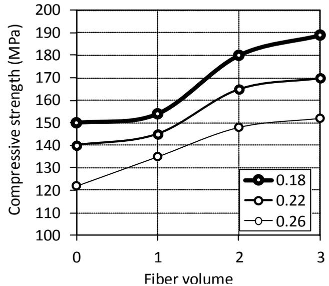
Fig. 7. Compressive strengths.
