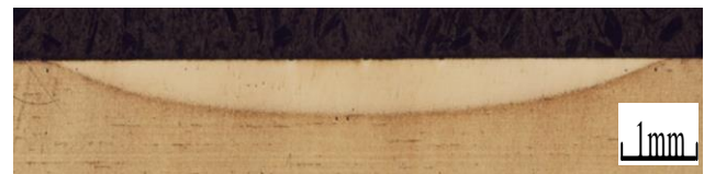
Fig. 8. Micrograph of the cross-sectional surface of CrAlN-coated specimen laser-irradiated at P=720 W.
